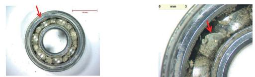
Upper bearing after removal of flanges, with 2 mm transluscent particle
