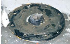
Top of the sensor after removal of the attachment plate (presence of yellow paint)
