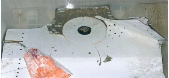
Angle of attack sensor attached to the aeroplane structure
