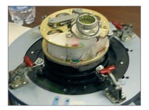
After the water was drained off and the electronic cards were dried in compressed air, the sensor was placed back in the chamber and the temperature was lowered to - 20 °C without the heating system being electrically powered. It was observed that the sensor blocked again.
