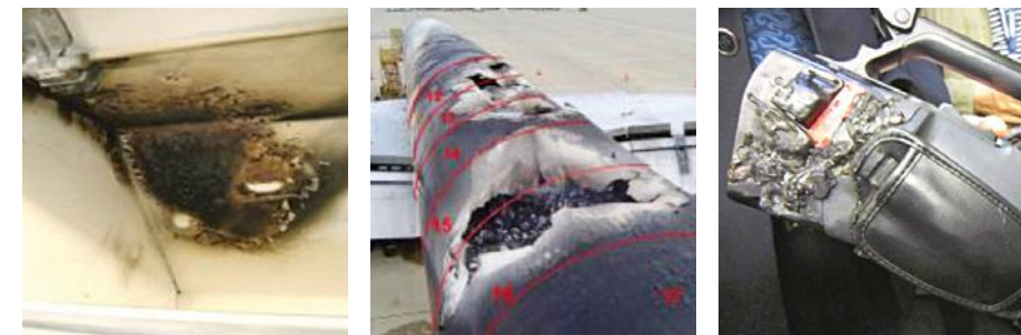
Damage to cabin overhead compartment video camera
