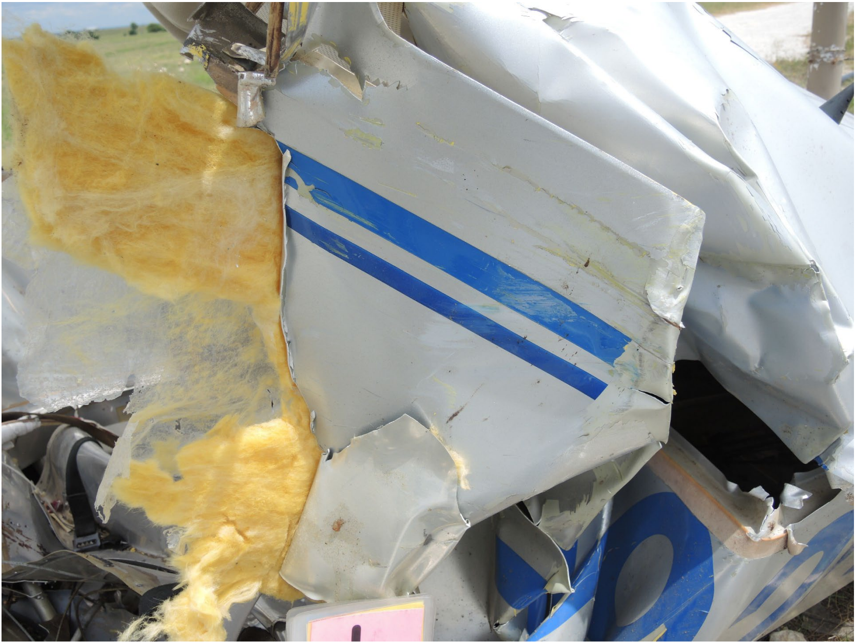
Photo 11 – Left Rear Fuselage Witness Marks
