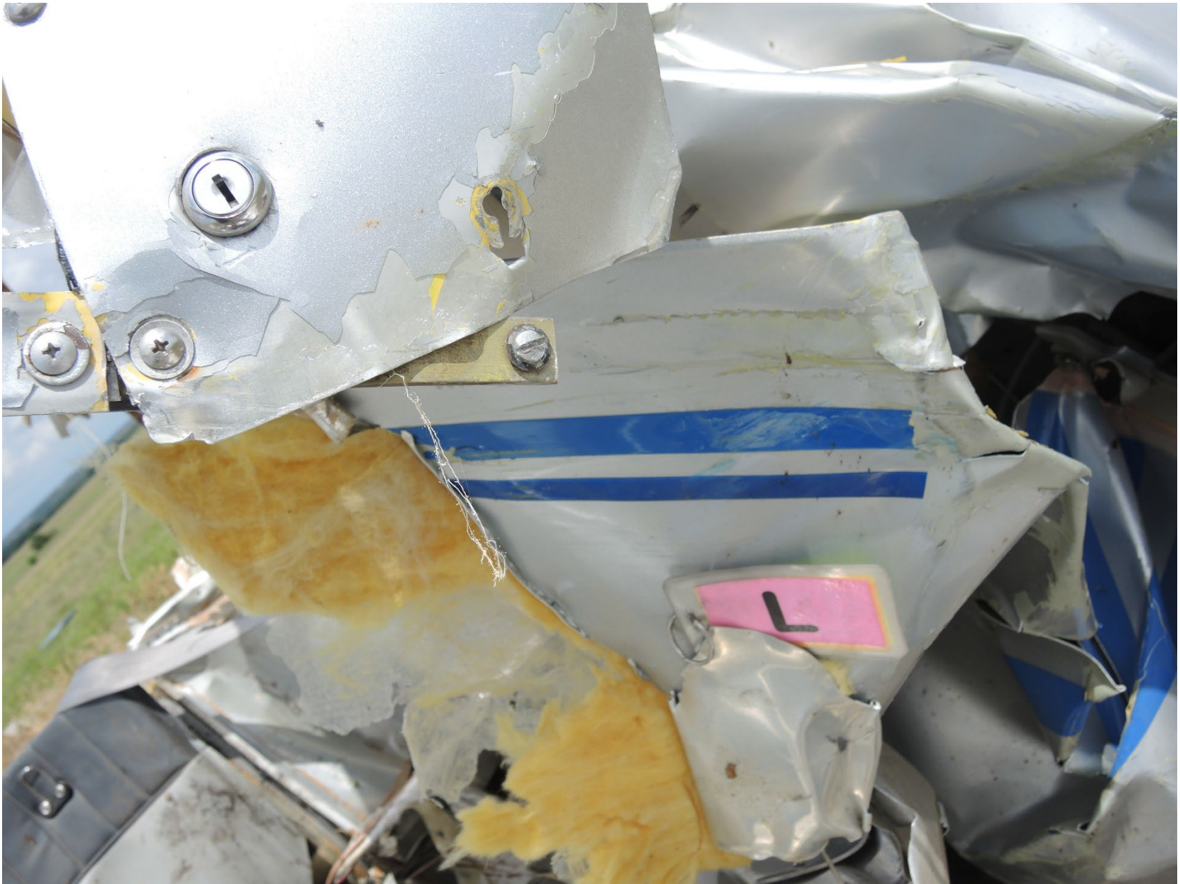
Photo 13 – Left Rear Fuselage Witness Marks
