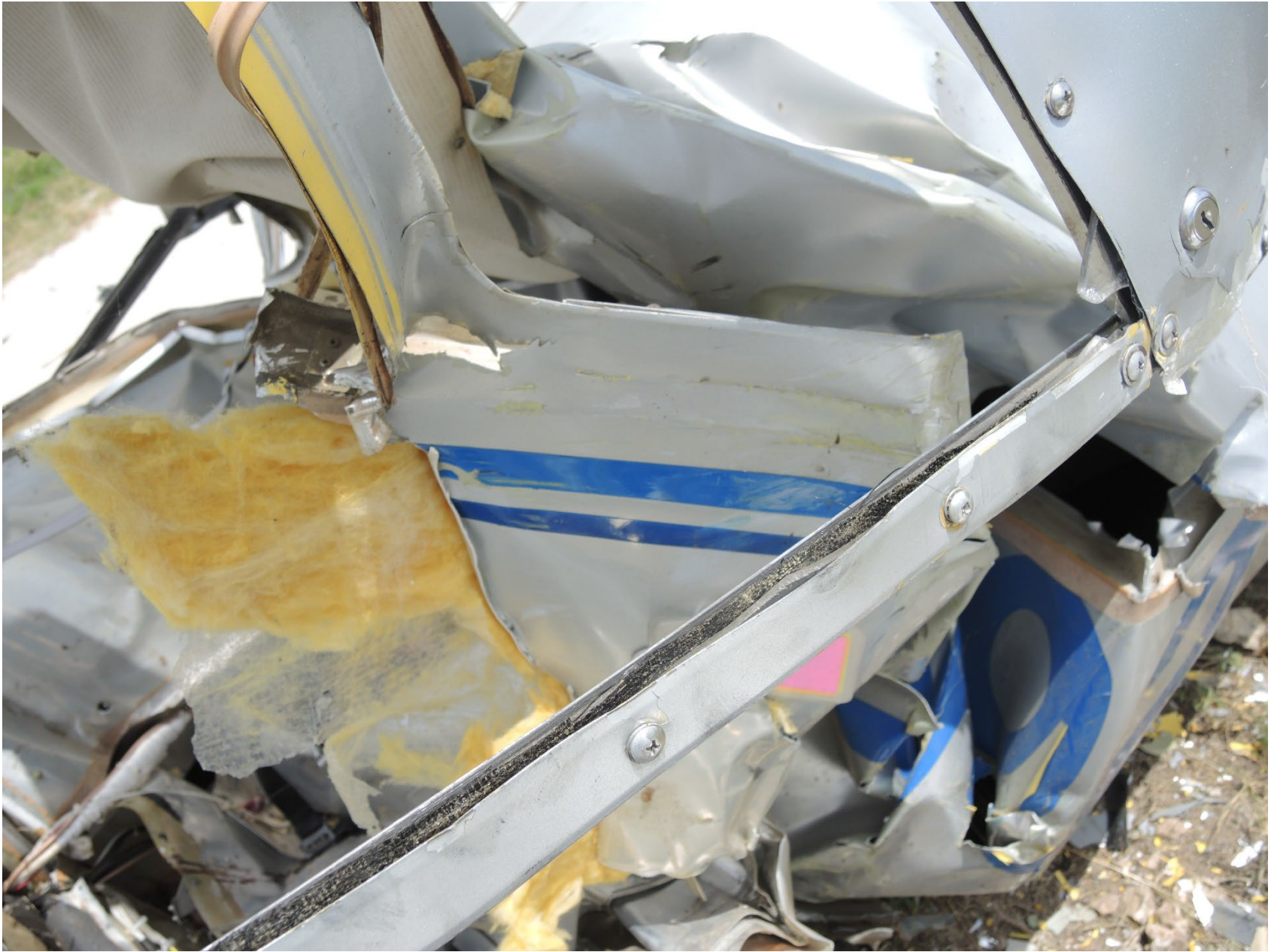
Photo 12 – Left Rear Fuselage Witness Marks
