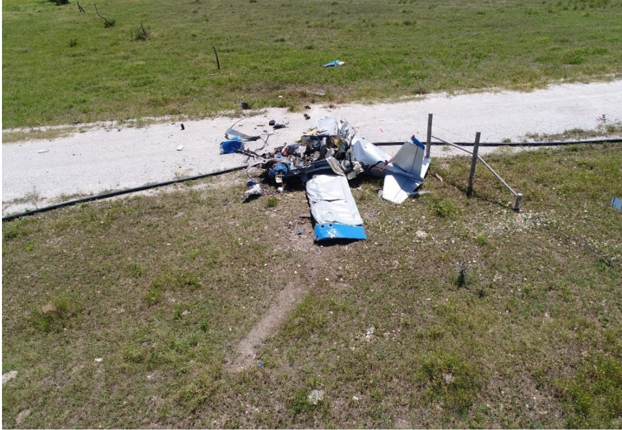
Figure 2. Aerial view of main wreckage. Left wing impact mark noted
