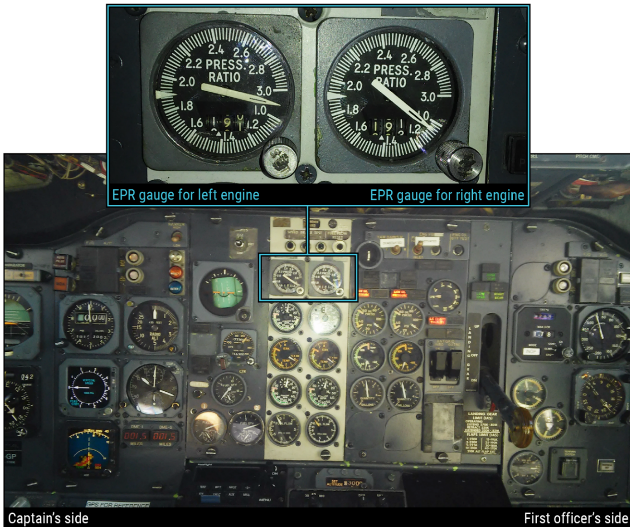
Figure 3. EPR gauges on the accident airplane’s center instrument panel (Source: Transair).
