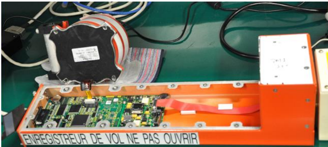
Figure 1.11-3 FDR CSMU connection to chassis
