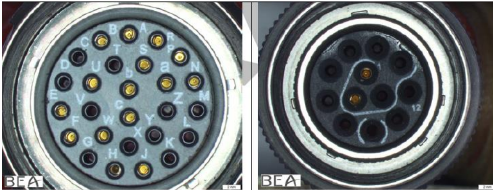
Figure 1.16-7 Connectors of AFU (left) and torque sensor (right)
