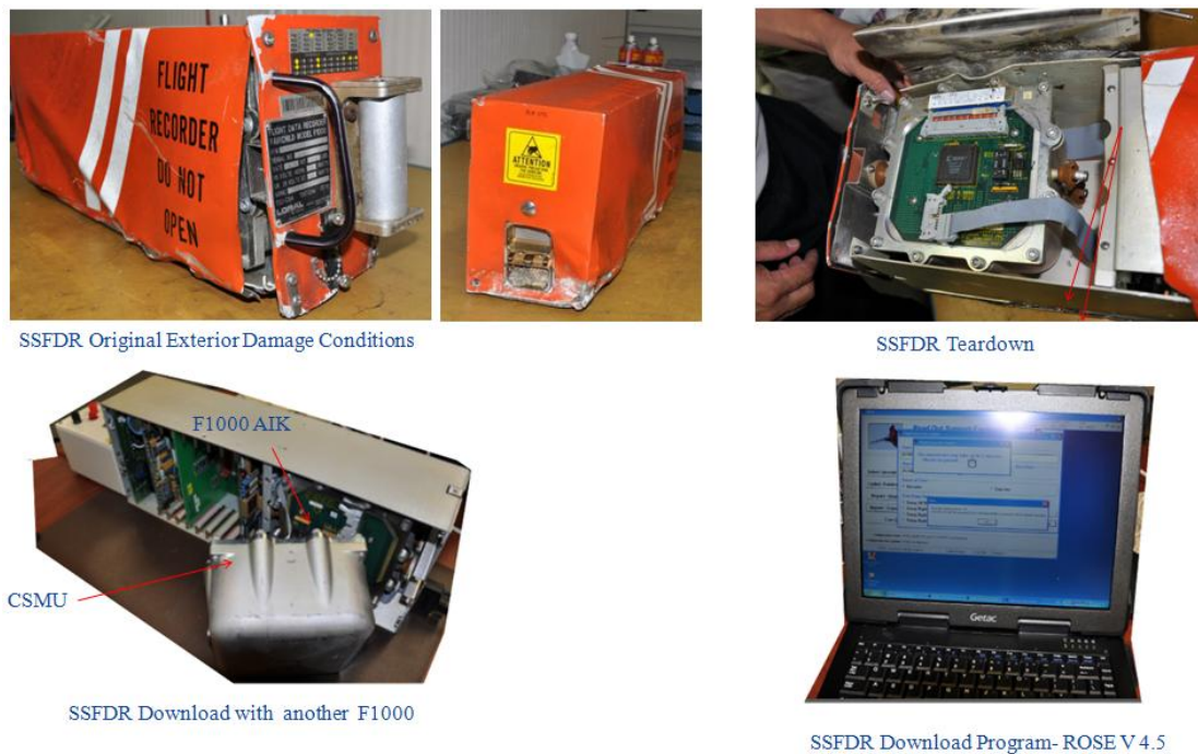
Figure 1.11-2 FDR exterior view, teardown and download process
