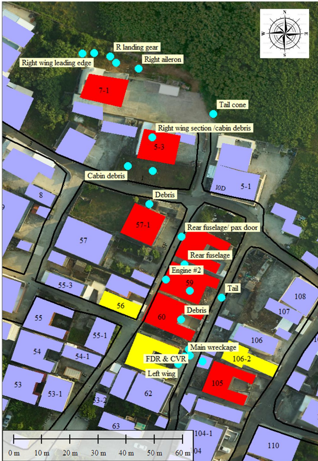
Figure 1.12-7 Wreckages distribution overlaid on Xixi village street map
