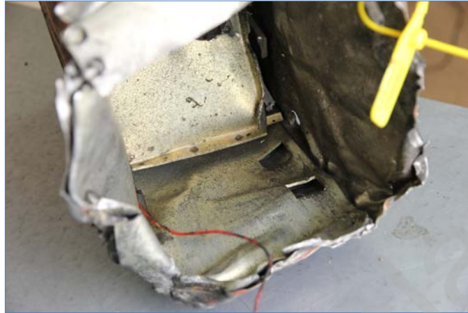
Figure 13 CVR housing without the memory unit
