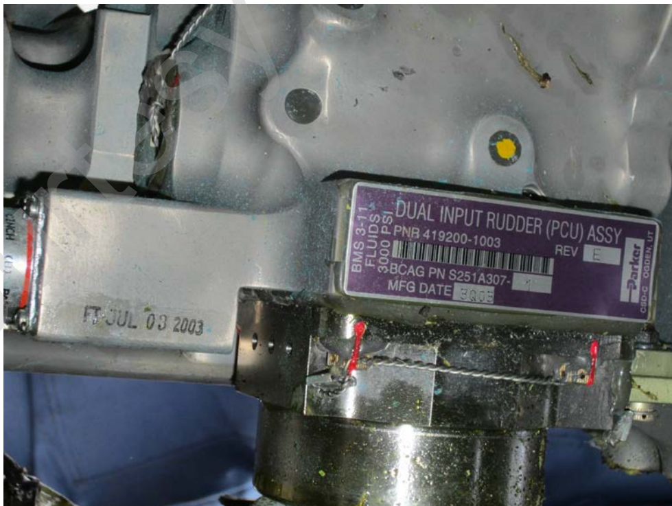
Figure 3 Main rudder PCU
