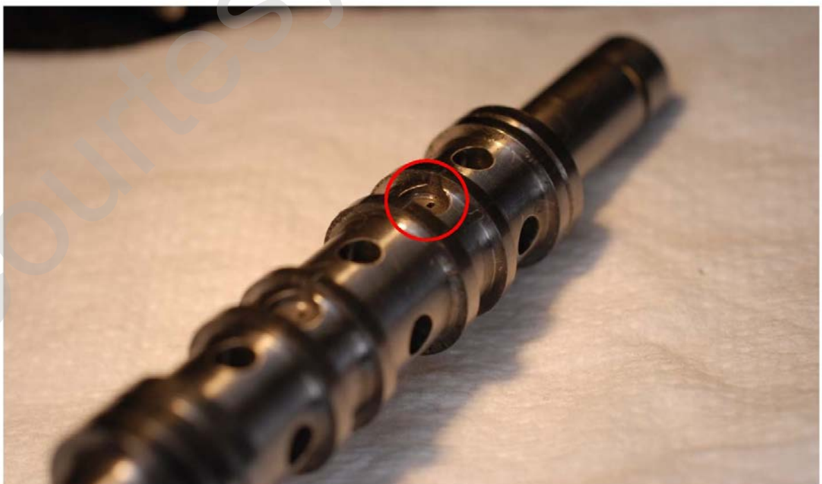
Figure 69 RH control valve secondary slide land edge deformation
