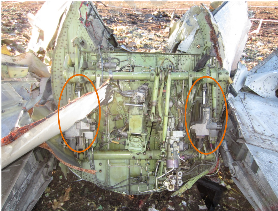
Figure 2 Appearance of frame 1156 on the air accident site (the elevators actuators are circled orange)
