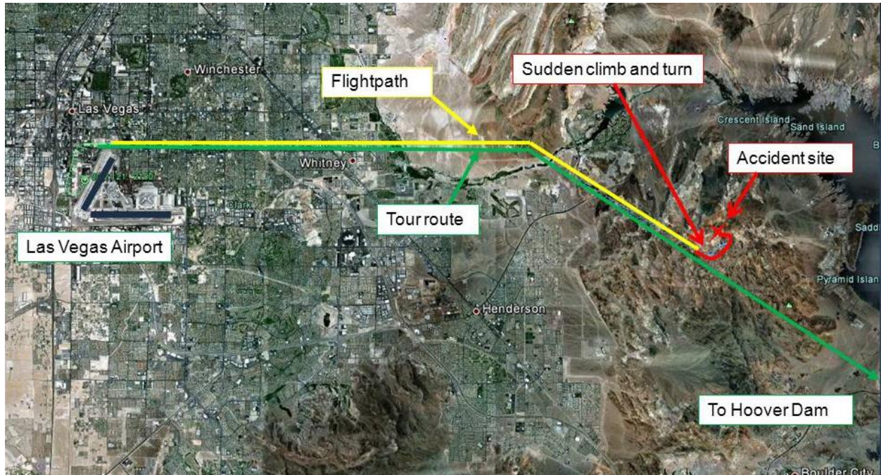
Figure 1. Accident flightpath (depicted in yellow) overlaid with the prescribed Twilight tour route (depicted in green).
