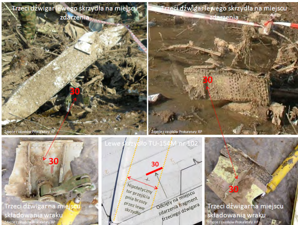
Fig. 15. View of the same part of spar no.3 from the detachable part of the left wing on the main crash site and place of storage of the debris.
