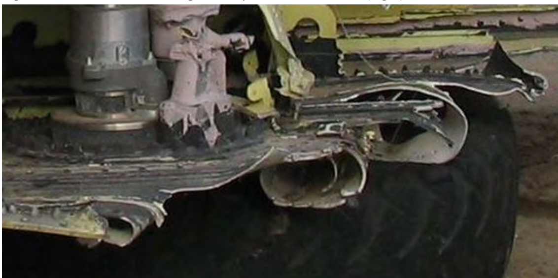
Fig. 2. Side view of the broken section of the left wing tip of TU-154M no.101 showing significant explosive signatures (curled edges of up to 450°).
