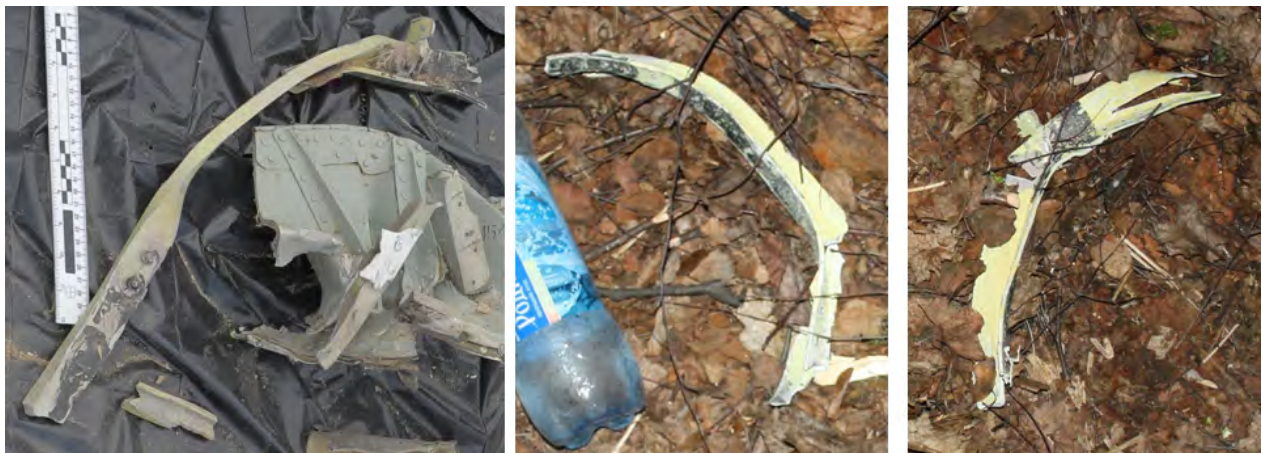
Fig.8. Pieces of stringers of the left wing curled outwards
