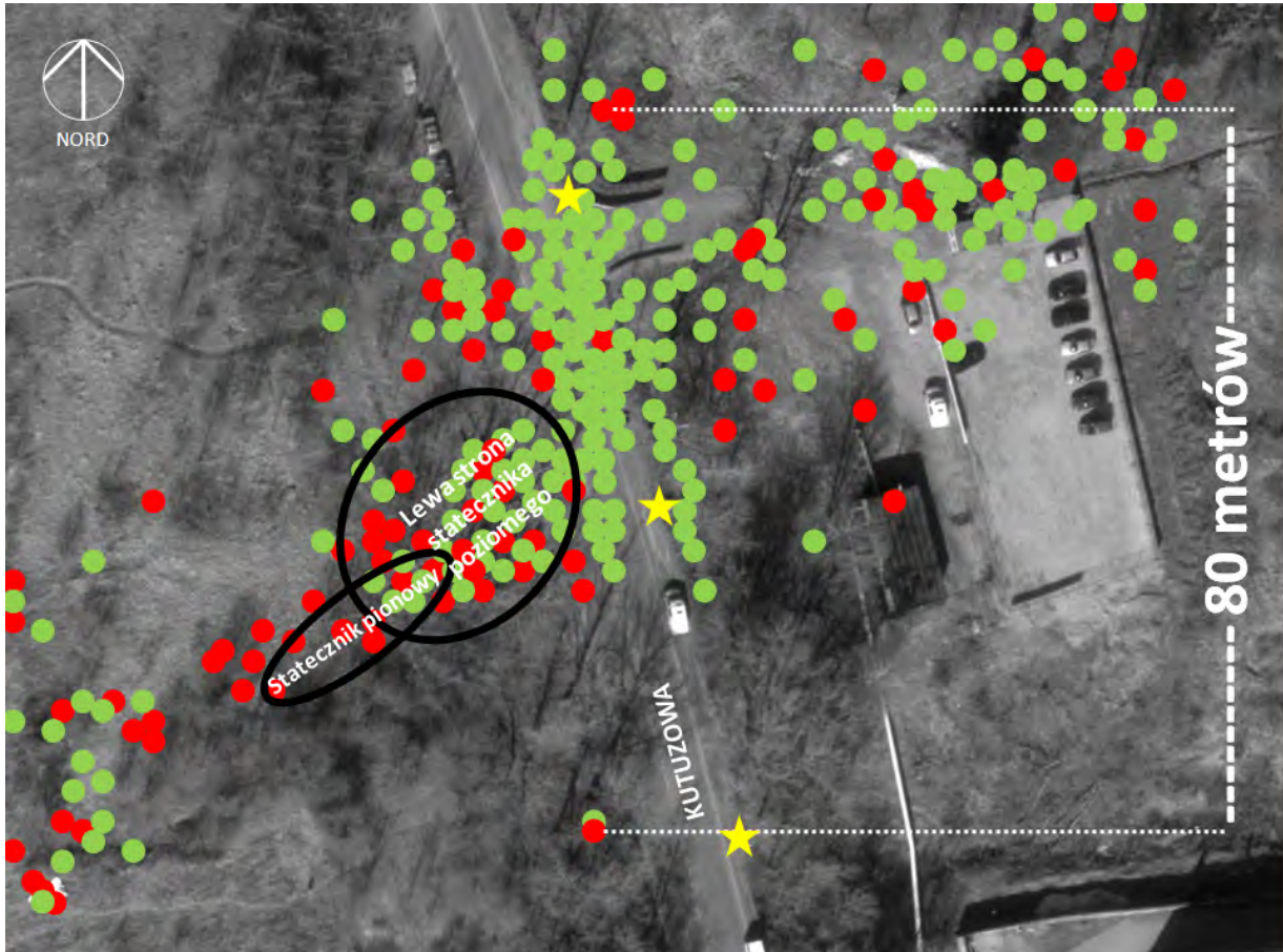
Fig. 27. Placing the left side of the horizontal stabilizer and the vertical stabilizer behind the Kutuzov highway. Flight direction is from right to left. Red dots show debris from the Tu-154M and green dots show debris from the associated tree damage.
