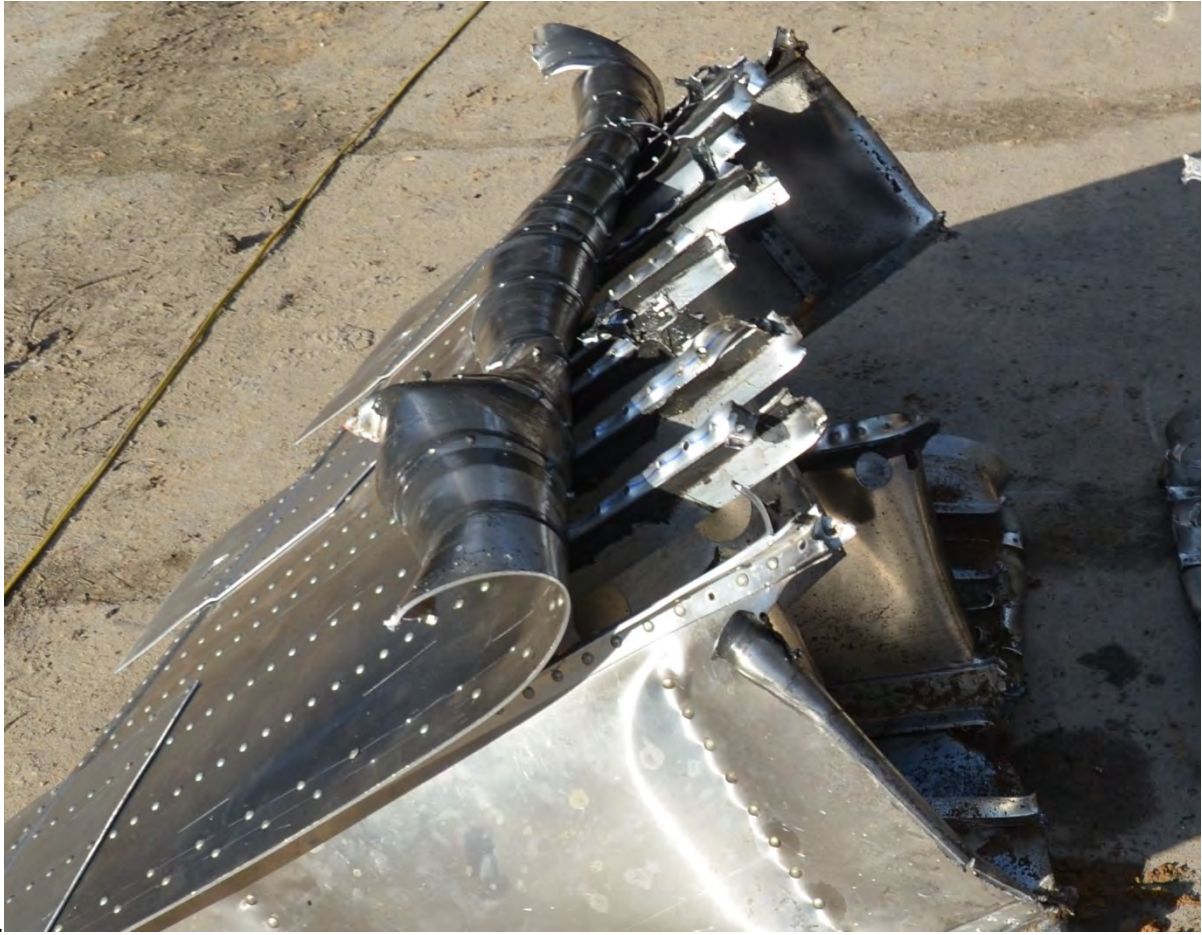
Fig. 23. Scale 1:1 Separation by explosive material of the wing box containing fuel. The experiment demonstrated the wing could be cut without a secondary major fuel explosion.
