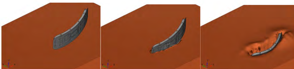
Figure 48 Shows results from NIAR's simulation of the door hitting soft ground and the door 1meter in the ground as Russians were digging it out by hand.
