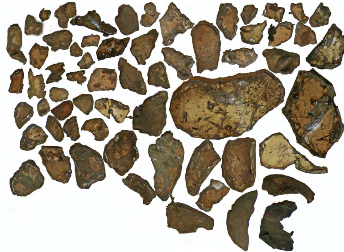
Fig. 33. Collected pieces of the Tu-154M taken from the ground 100m before the main crash site showing thermal traces.
