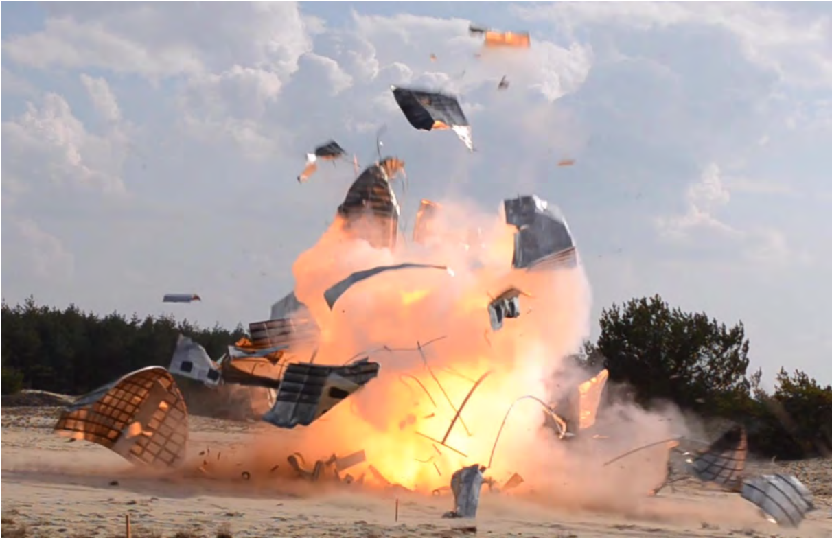
Fig. 52. Explosion of a thermo-baric charge in the occupant's part of the fuselage resulting in the complete destruction of the fuselage and the formation of much small debris.
