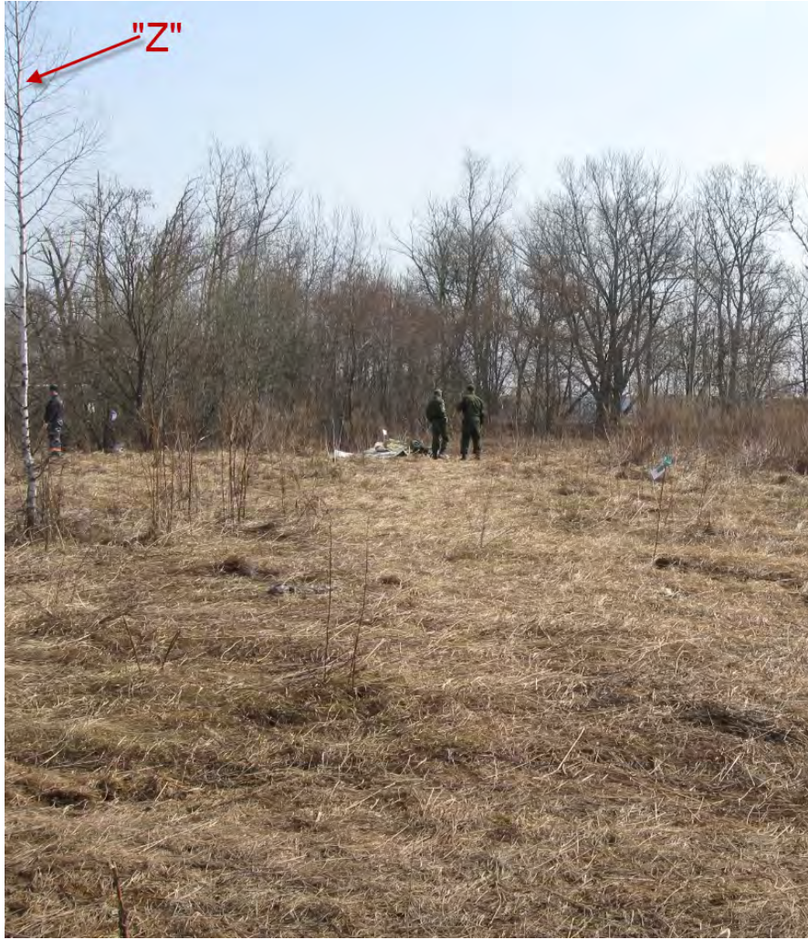
Fig. 30. The tree marked "Z" growing in the direct vicinity of the flight path, when the plane is flying from the Kutuzov Street (in the background) to the place of crash. On the right side starting at the blue marker on a stick there is a visible ground trace when hitting the ground with the left stabilizer.
