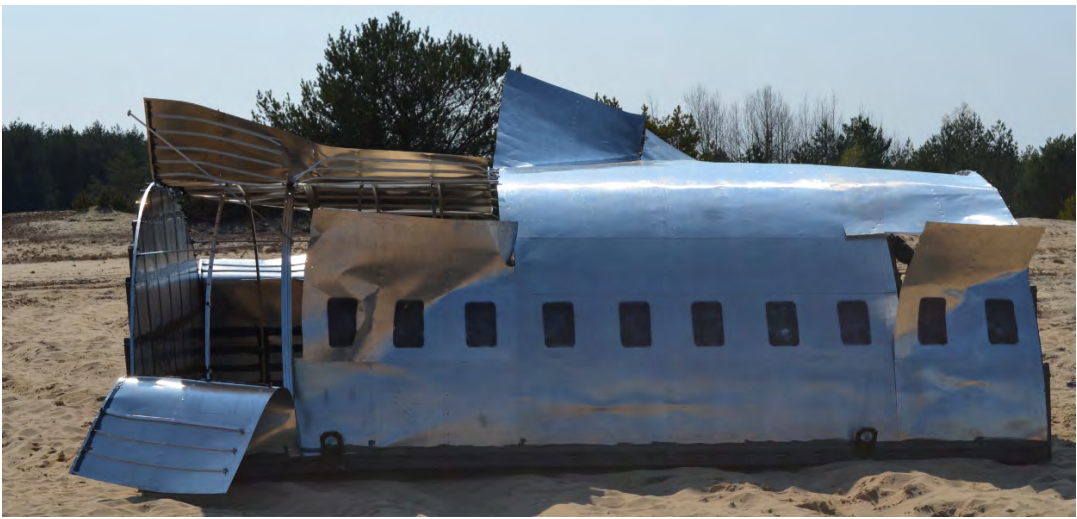
Fig.51. Explosion of jet-fuel in the occupant's part of the fuselage resulting in a large opening but no destruction in small pieces.
