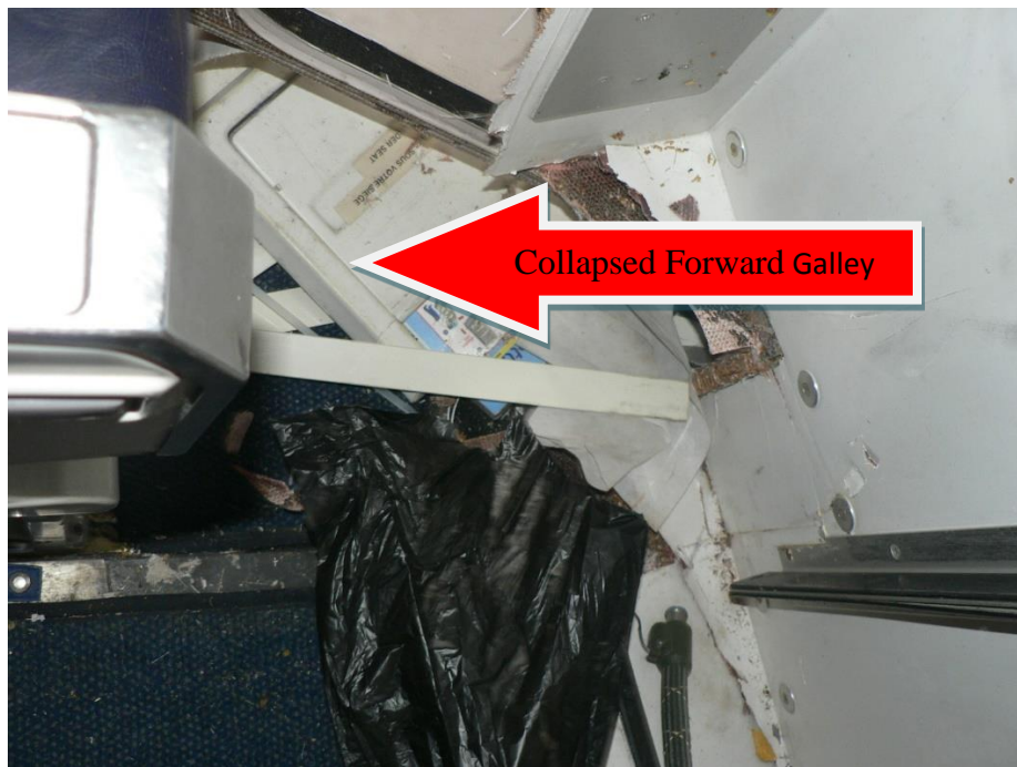
Photo 5. View of Collapsed Forward Galley
