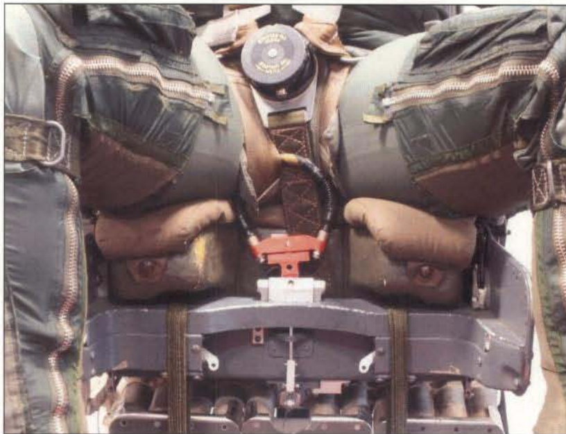
Figure 21 – Incorrect routing of RH crotch strap through SFH.
