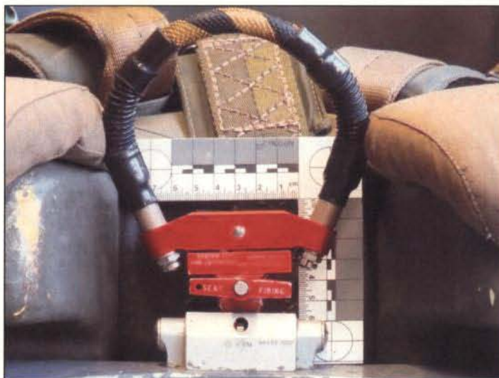
Figure 23 – SFH safety pin fitted whilst SFH remains in an unsafe condition.
