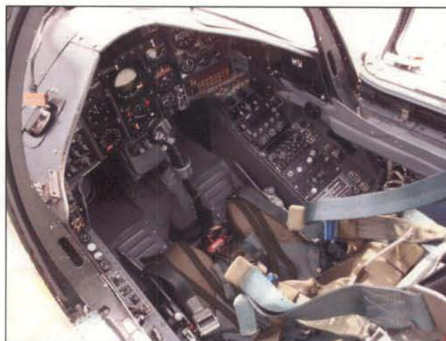
Figure 26 – SFH viewed from above; seat motored to the lower limit.
