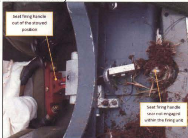
Figure 9 – XX177 SFH out of housing and sear not engaged.
