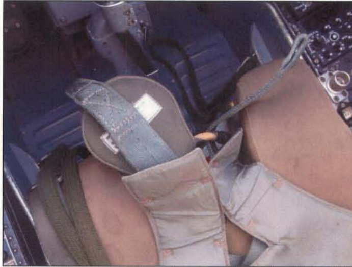
Figure 20 – Straps moved off seat obscuring SFH prior to crew cockpit entry with the RH crotch strap miss-routed through the SFH.
