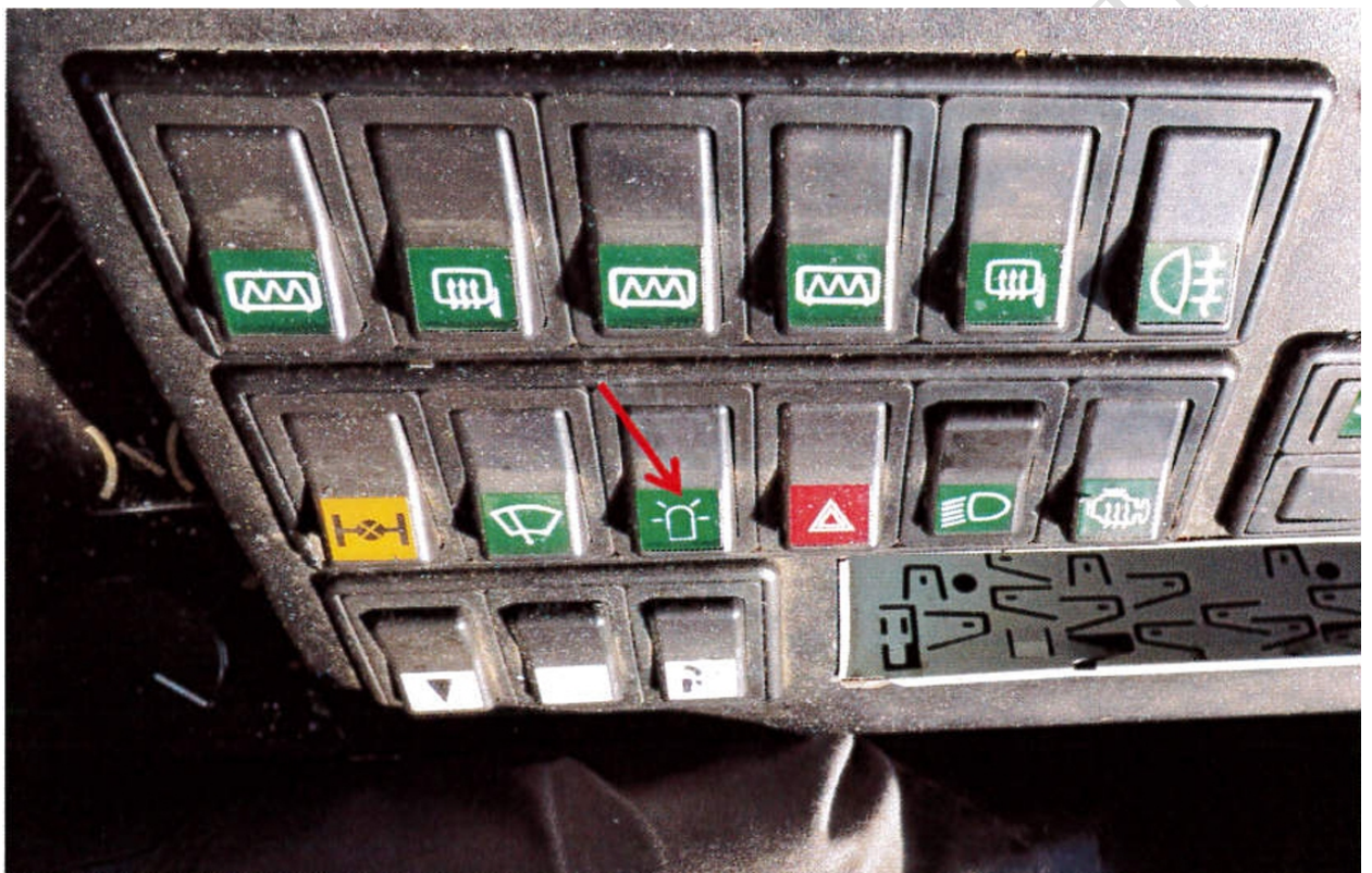
Figure 53. Strobe lights activation switch (marked with an arrow) on the cab control panel in the SCHMIDT SUPRA-5001, state number 377
