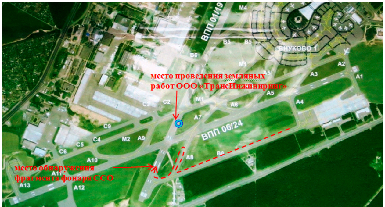
Figure 59. Vehicle path (shown in dotted line) after snowplow 2 was broken and before snowplow 1 detected the fragment of runway light
