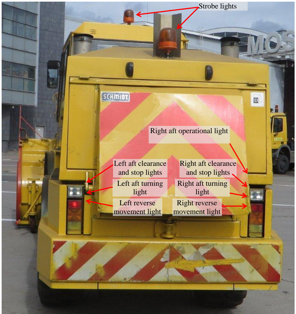
Figure 46c. Snowplow lights schematic (aft)
