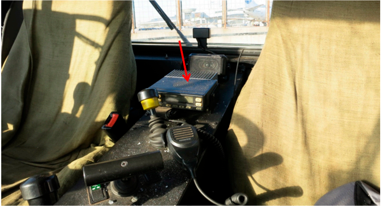
Figure 54. Kenwood radio station in the cab of SCHMIDT SUPRA-5001, state number 377 (marked by the arrow)
