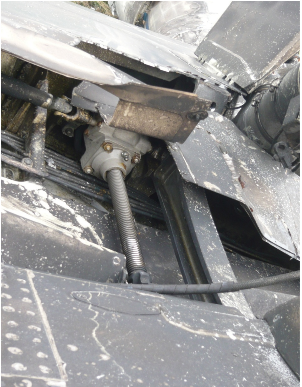
Figure 43. Flaps actuator jack screw
