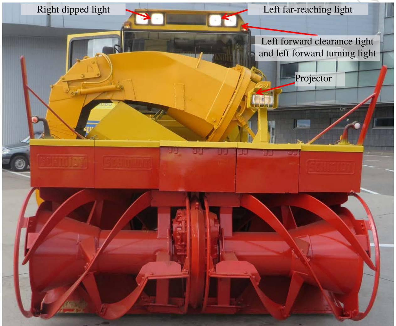
Figure 46b. Snowplow lights schematic (forward)
