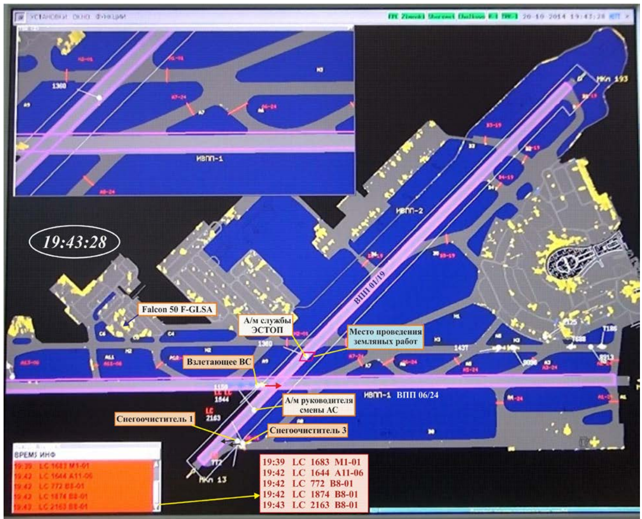
Figure 94. TRADIS indicator on departure controller's WP at 19:43:28 (light red table shows information in the alert list)
