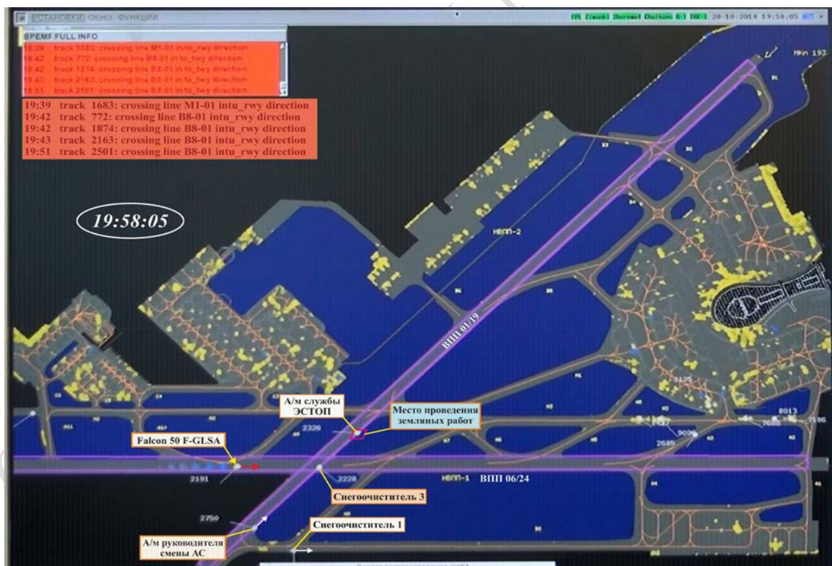
Figure 13. TRADIS indicator on ground controller's working position before the accident with additional information from the investigation team
