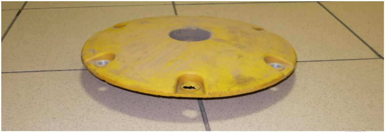
Figure 58. Fragment of runway light (basement)
