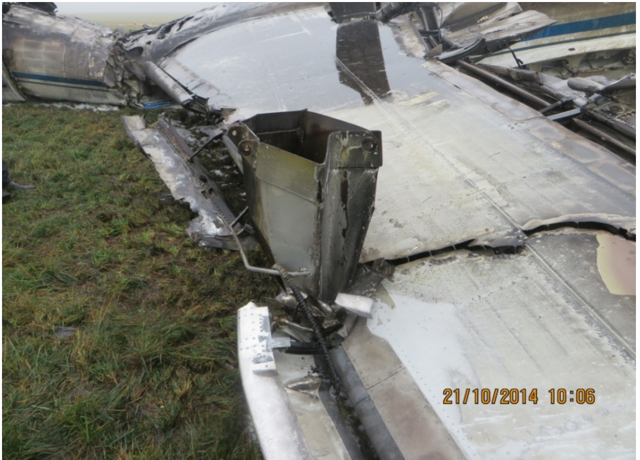
Figure 39. RH wing with a snowplow fragment
