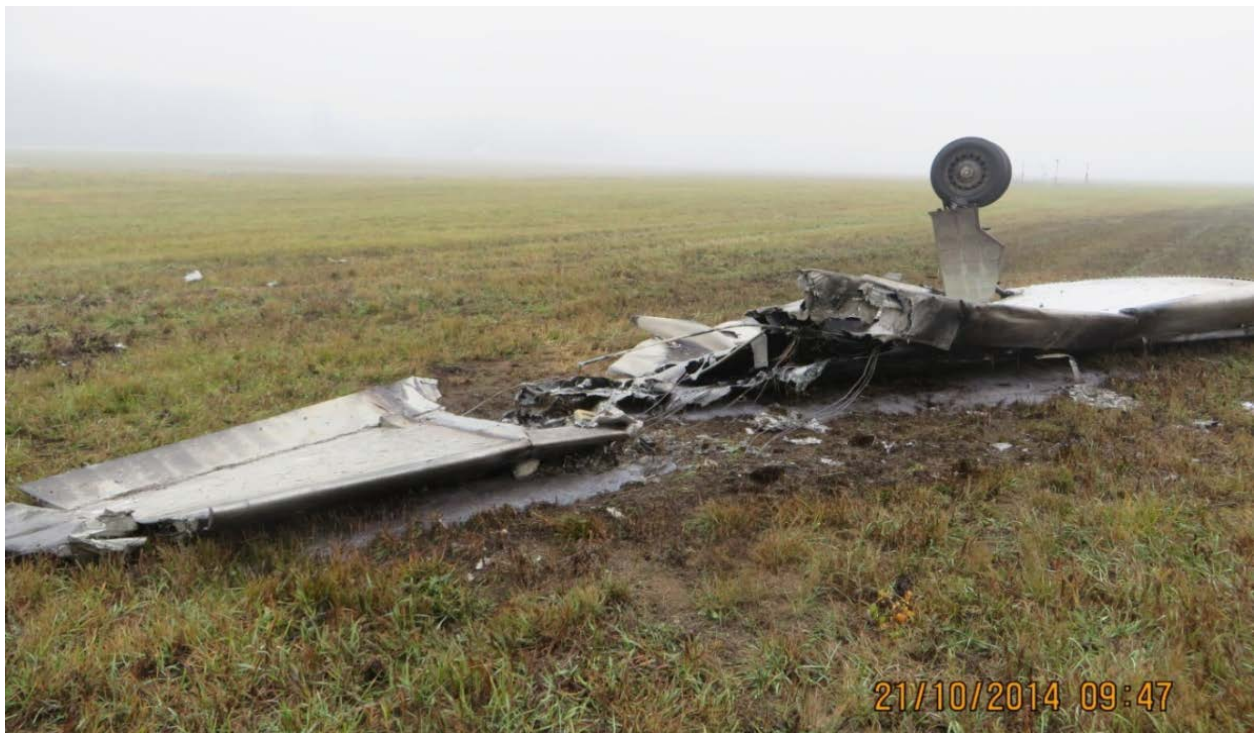
Figure 41. LH wing with LH main landing gear
