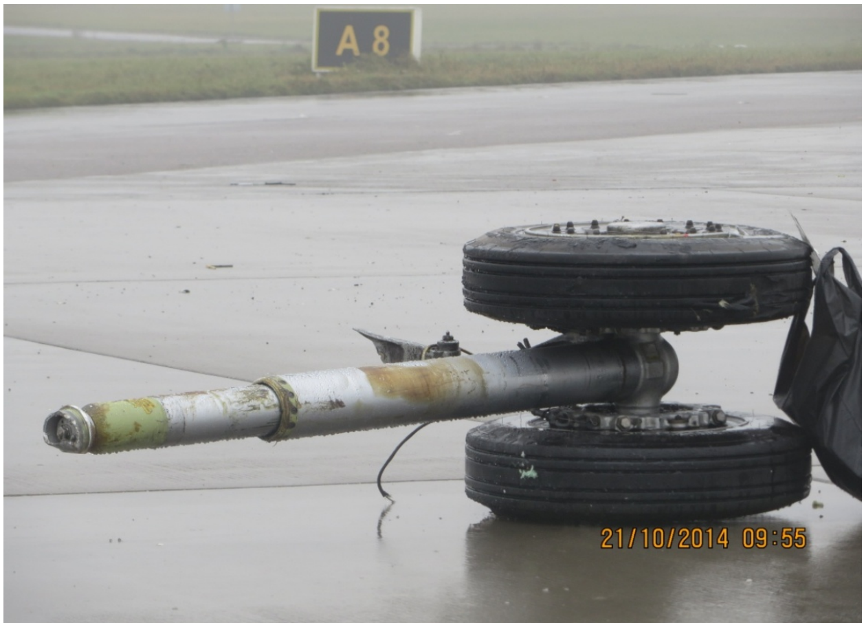
Figure 46. RH main landing gear
