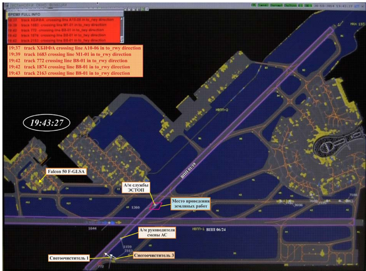
Figure 57. Location of objects at airdrome Vnukovo as viewed from the ground controller screen at 19:43:27
