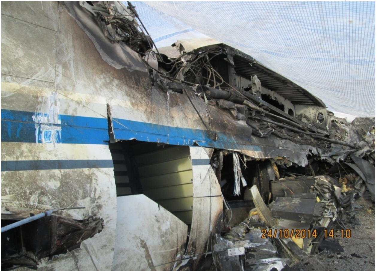
Figure 38. Fuselage and LH wing attachment
