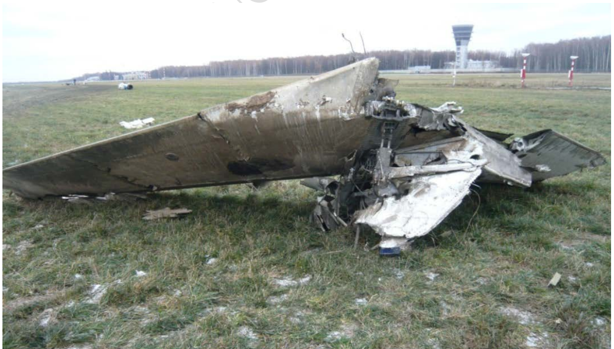
Figure 42. Fragment of fin with horizontal stabilizer
