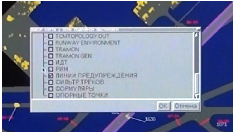
Figure 22. Technical chart status with Reserved Lines at Supervisor WP. The chart is activated (ticked)
