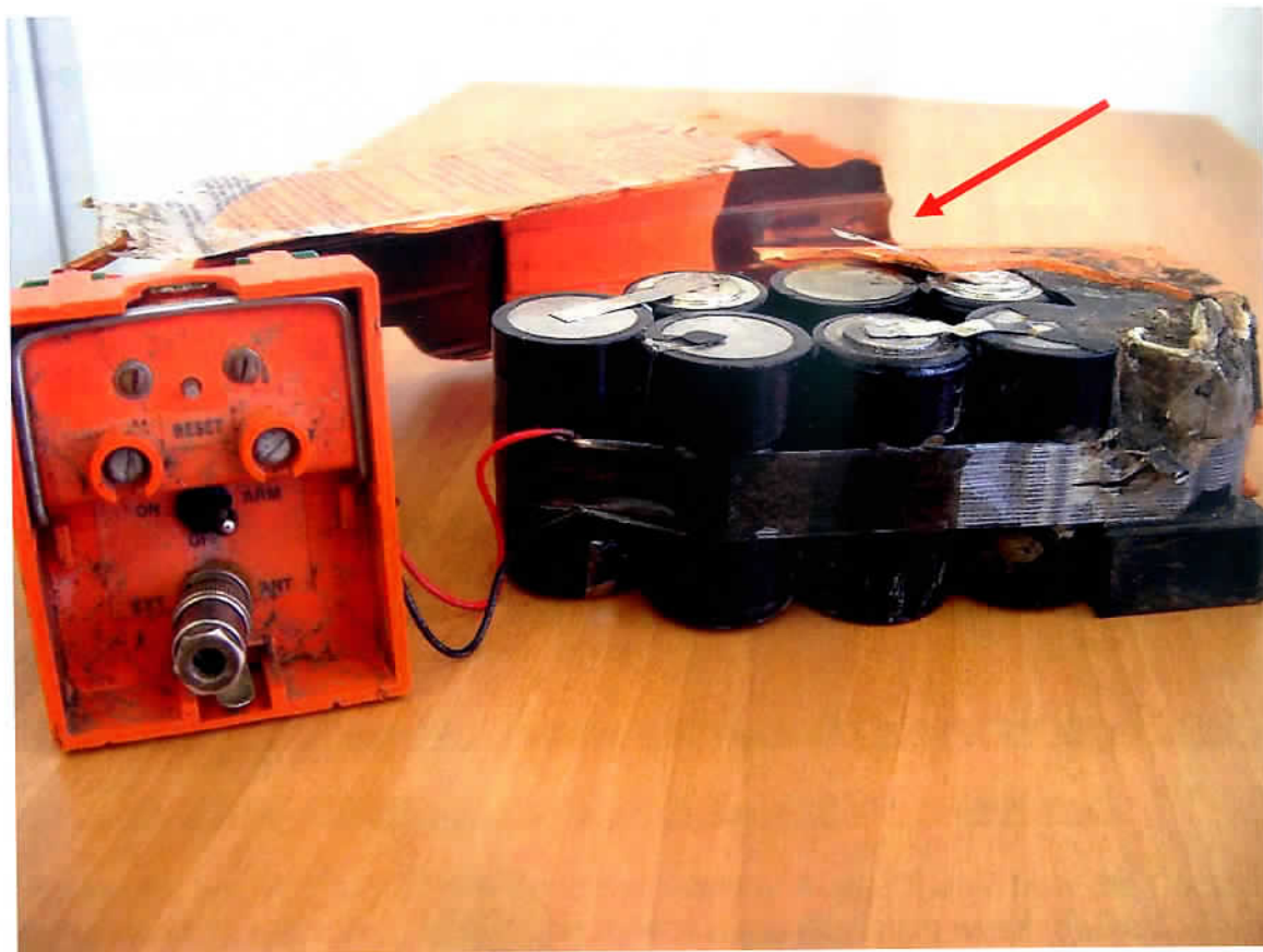
Picture 8.24: ELT batteries loose connection
