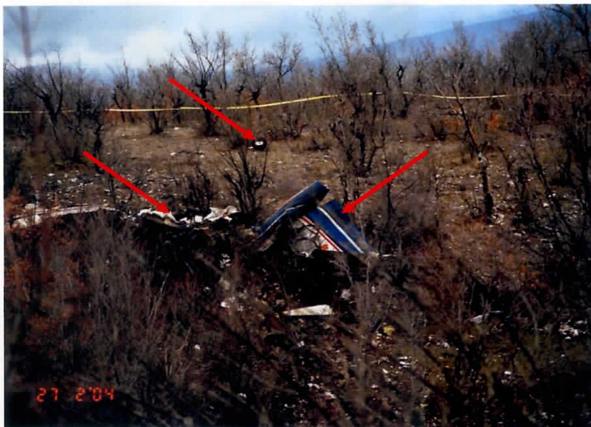
Picture 8.13: Tail unit, left wing, left engine and wheel at the resting place
