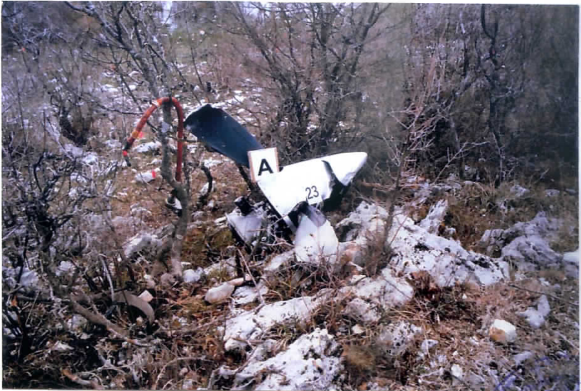
Picture 8.8: Right propeller and associated reduction gear box
