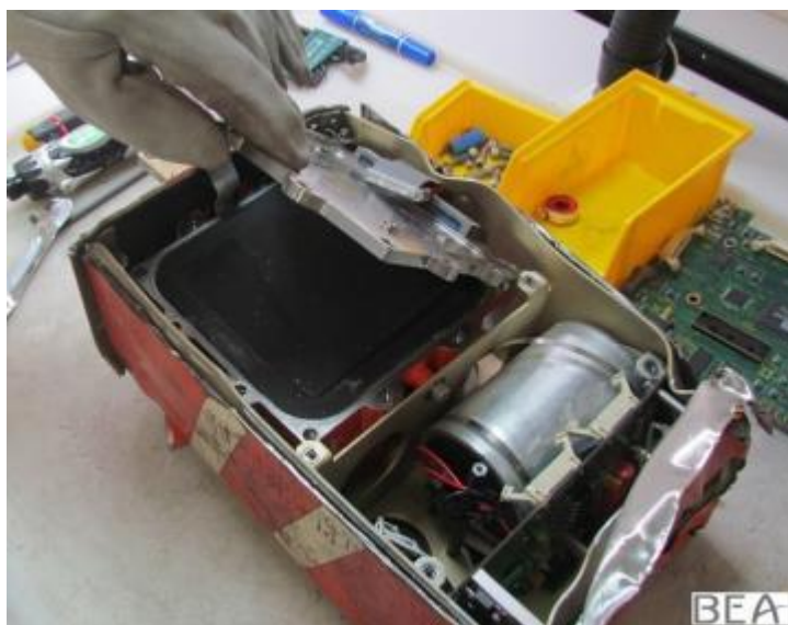
The FCSSU was opened and the metallic casing was extracted from the recorder.
