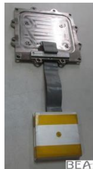
The FCSSU was opened and the metallic casing was extracted from the recorder.
