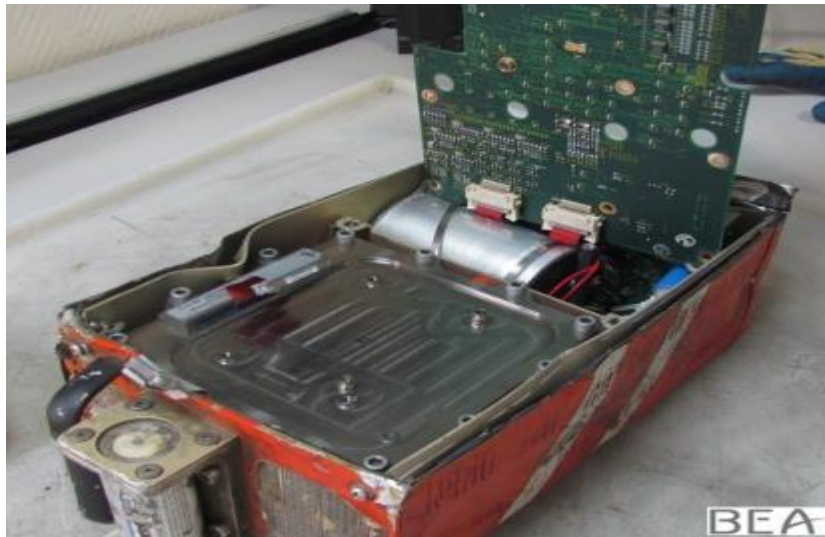
The FCSSU was opened and the metallic casing was extracted from the recorder.
