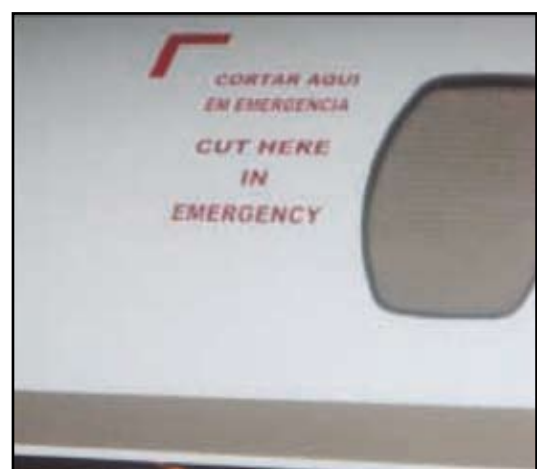
Emergency cutting area on aircraft fuselage
