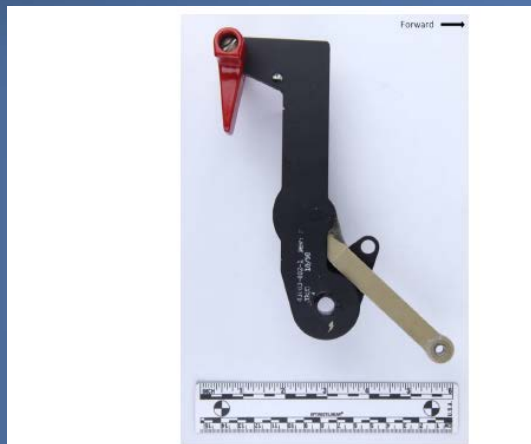
Figure 4a. Photograph of an exemplar gust lock handle in the ON position.
