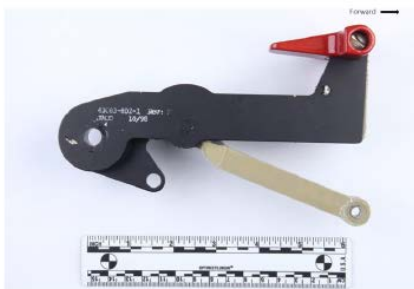
Figure 4b. Photograph of an exemplar gust lock handle in the OFF position.
