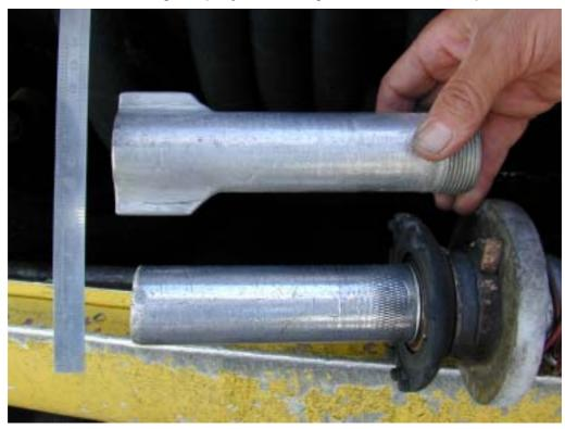
The delivery nozzle with enlarged outer diameter cannot be inserted into the tank openings of HB-LTC as these were modified to smaller diameters using metal plates.
