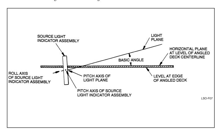
Figure 4-7. Determination of Basic Angle
