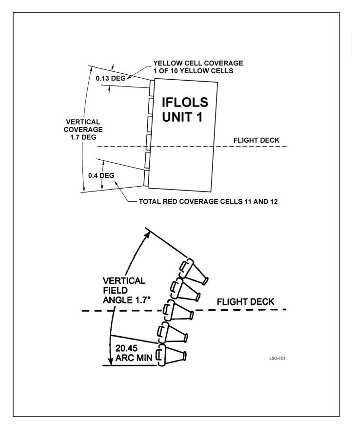
Figure 3-1. FLOLS Vertical Field Angle
