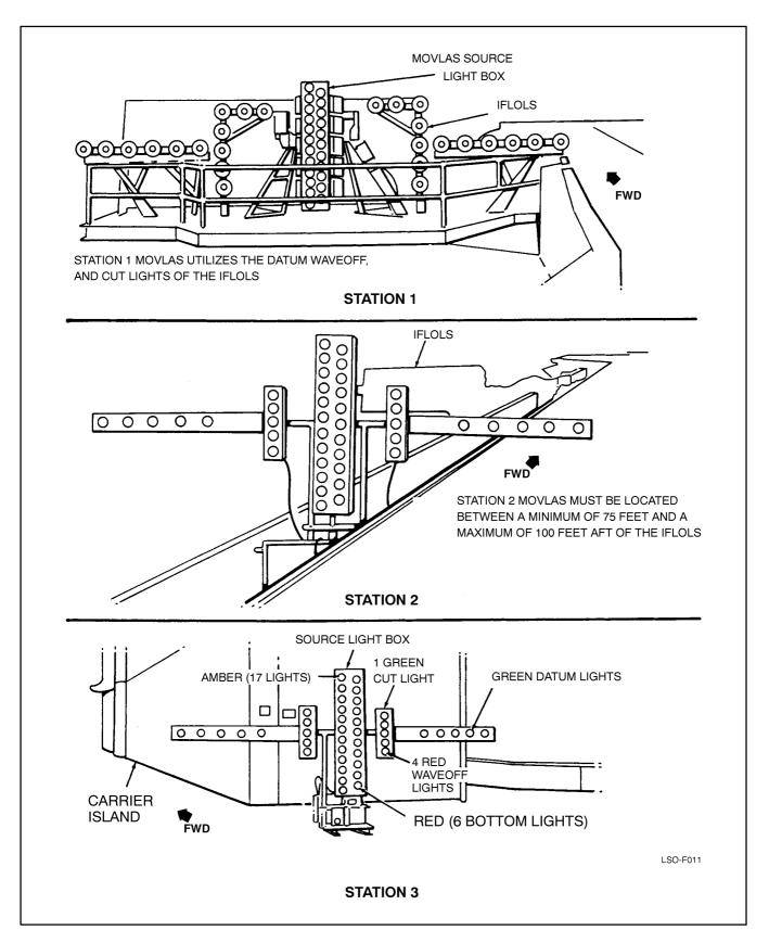
Figure 4-11. Manually Operated Visual Landing Aid System (MOVLAS) Mk 1 Mod 2 Shipboard, General Arrangement
