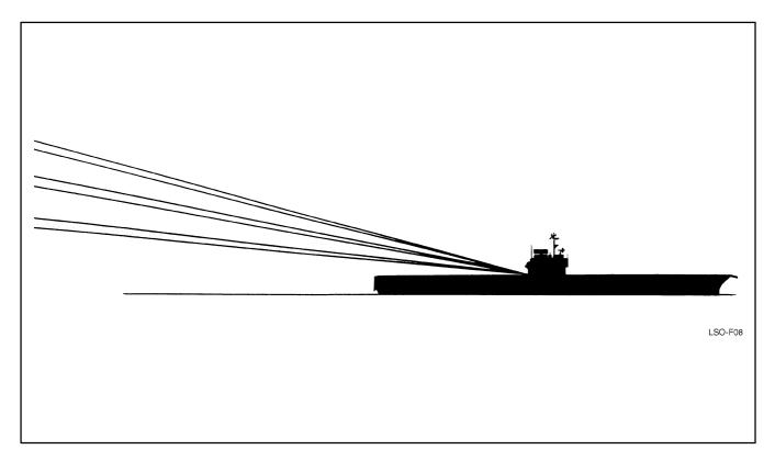
Figure 4-8. Effects of Pitch Angle (Basic Angle) Changes on Light Plane
