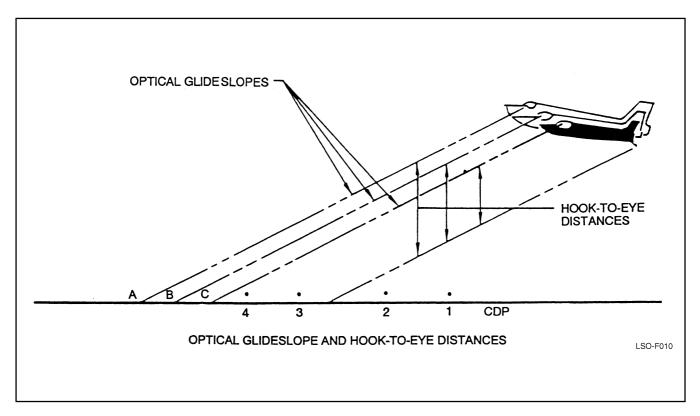
Figure 4-10. Optical Glideslope and Hook-to-Eye Distances
