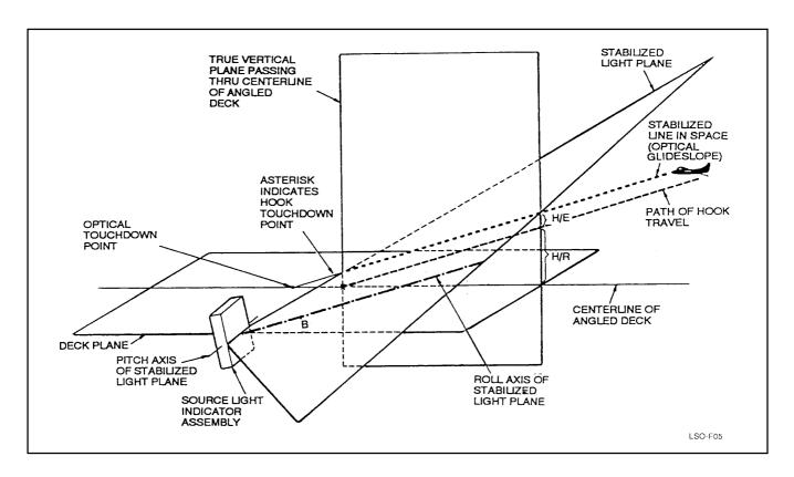
Figure 4-5. Geometry of Line Mode Stabilization
