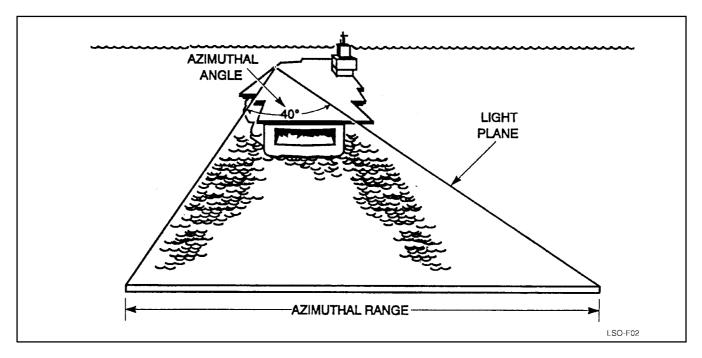
Figure 4-3. IFLOLS Azimuthal Range and Angle
