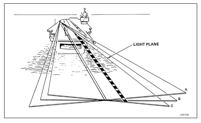
Figure 4-9. Effects of Hook-to-Eye Changes on Light Plane
