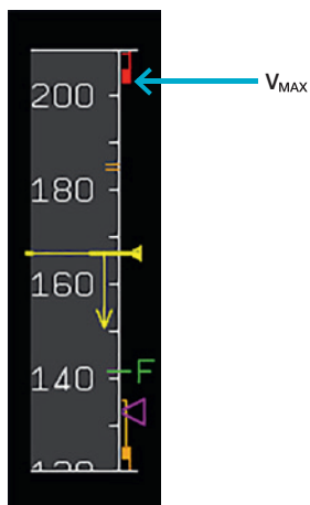
(fig.4) V MAX speed on the PFD speed scale
