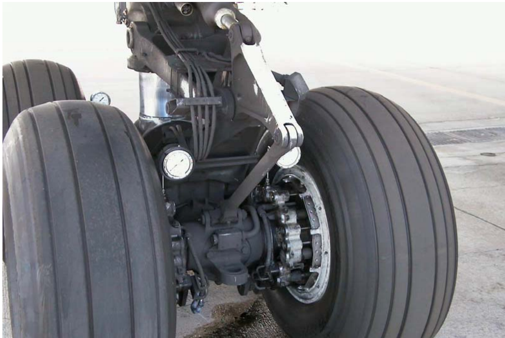
Gauges installed on the brakes of TF-ATH
