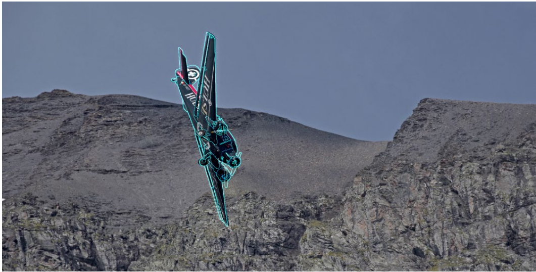
Figure 7: Image showing HB-HOT at point F16, including a superimposed three-dimensional model of an identical Ju 53/3m g4e (light blue) for the purpose of determining attitudes, wing deflection and deflections of the control surfaces. The direction of view is north-eastwards, the southern spur of Piz Segnas is visible in the background.
