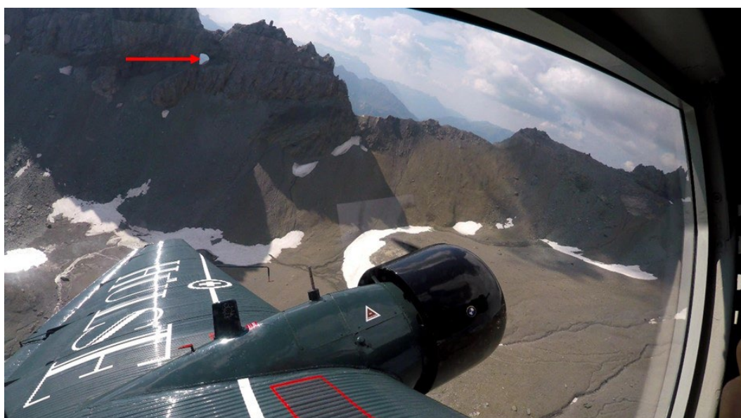
Figure 4: Still image from a video at point F13, recorded from the cabin of HB-HOT looking towards the Martinsloch (red arrow), 4.3 seconds after the image shown in figure 3 was taken. The pitch attitude was 12.1 degrees, the left bank attitude 32.7 degrees and the altitude 2,724 m AMSL.
