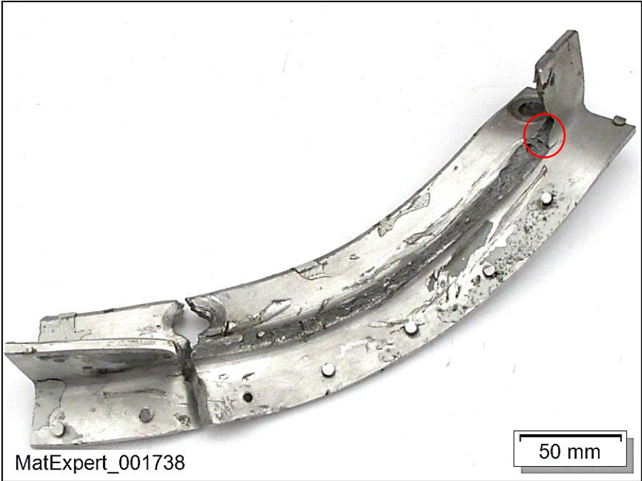
Figure 34: Location of the analysed fracture surface (red circle).
