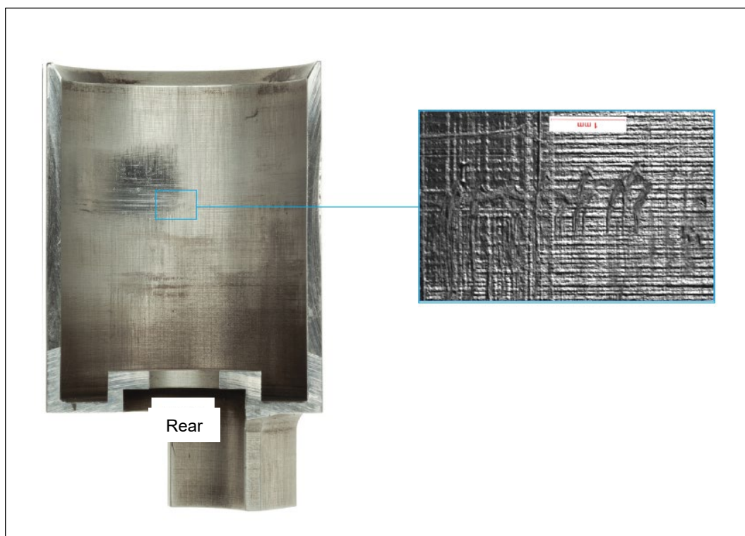
Figure 94: Abrasions in the pump cylinder from the carburettor for the centre engine.
