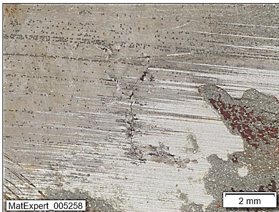
Figure 28: Area around joint 15 – brittle cracking, partially intergranular.
