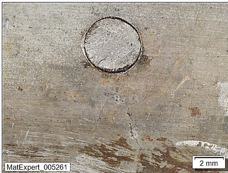
Figure 29: Area around joint 15 – brittle cracking, partially intergranular.
