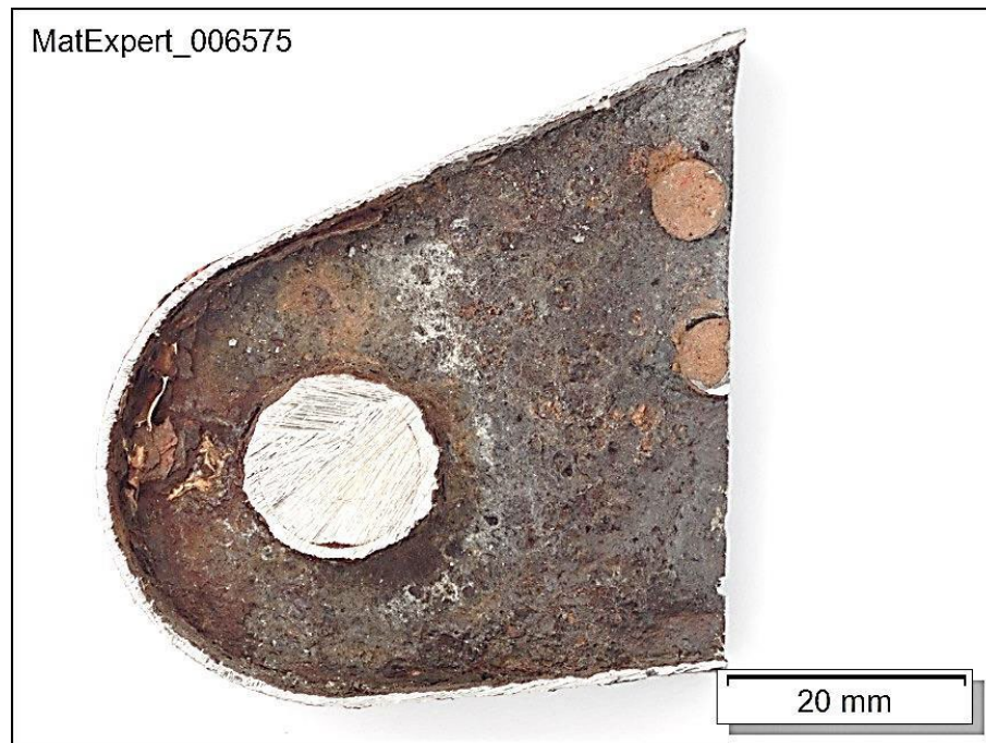
Figure 65: Severely corroded inner side of the cargo door hinge.
