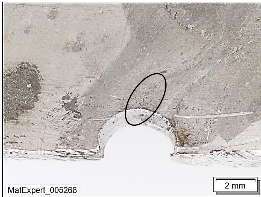
Figure 31: Close-up of figure 30 – start of a crack at the rivet hole (circled).
