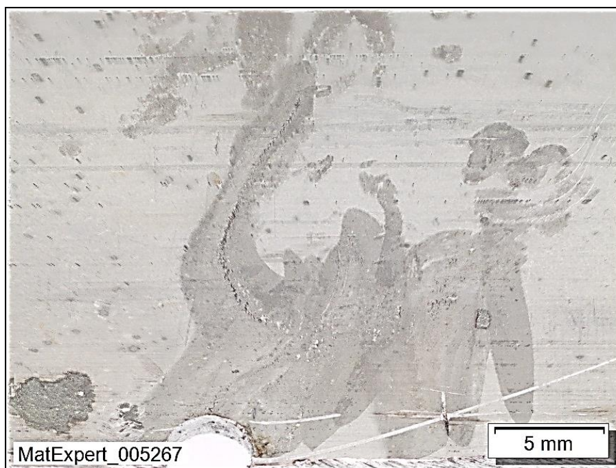
Figure 30: Area around joint 15 – crack-like surface condition.
