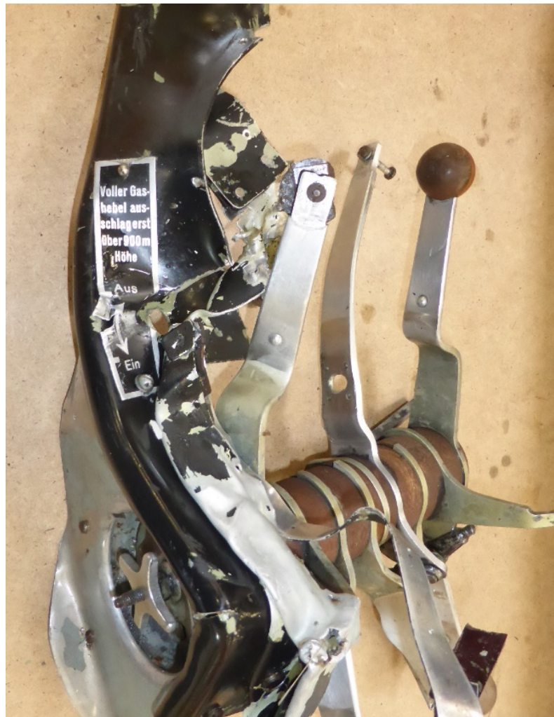
Figure 86: Deformed main throttle levers.
