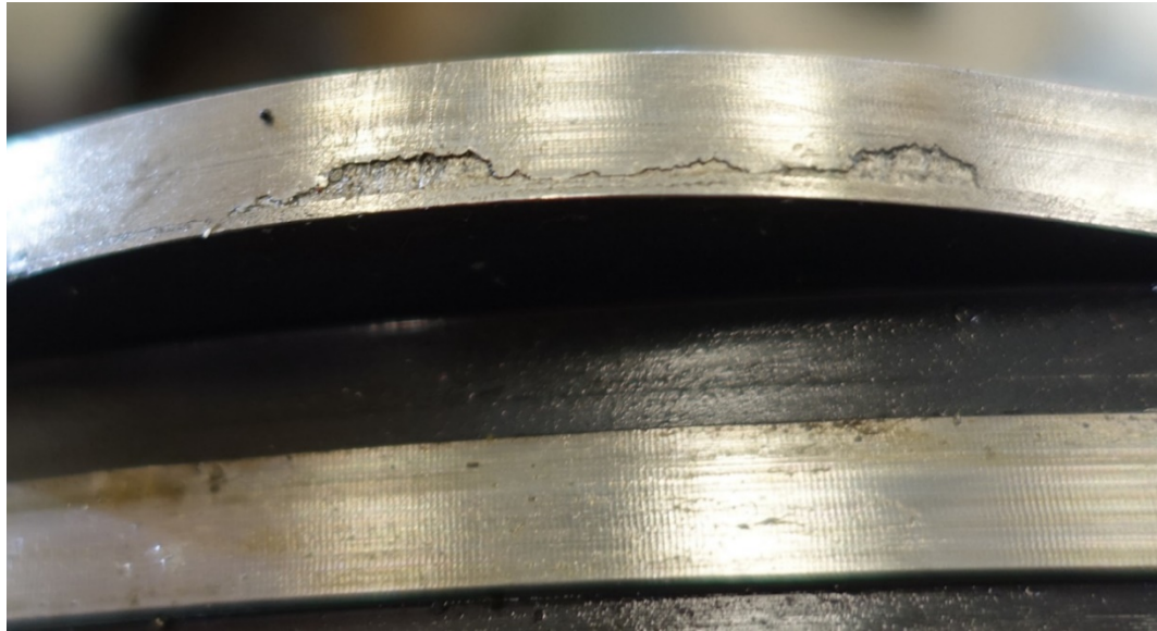
Figure 27: Cam discs from the centre engine – the machining marks (regular, finely grooved surface) and the chipping on the upper running surface are clearly visible.
