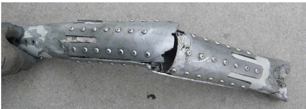
Figure 23: Tubular strut from the centre engine frame repaired with a doubler (see annex A1.6 ).
