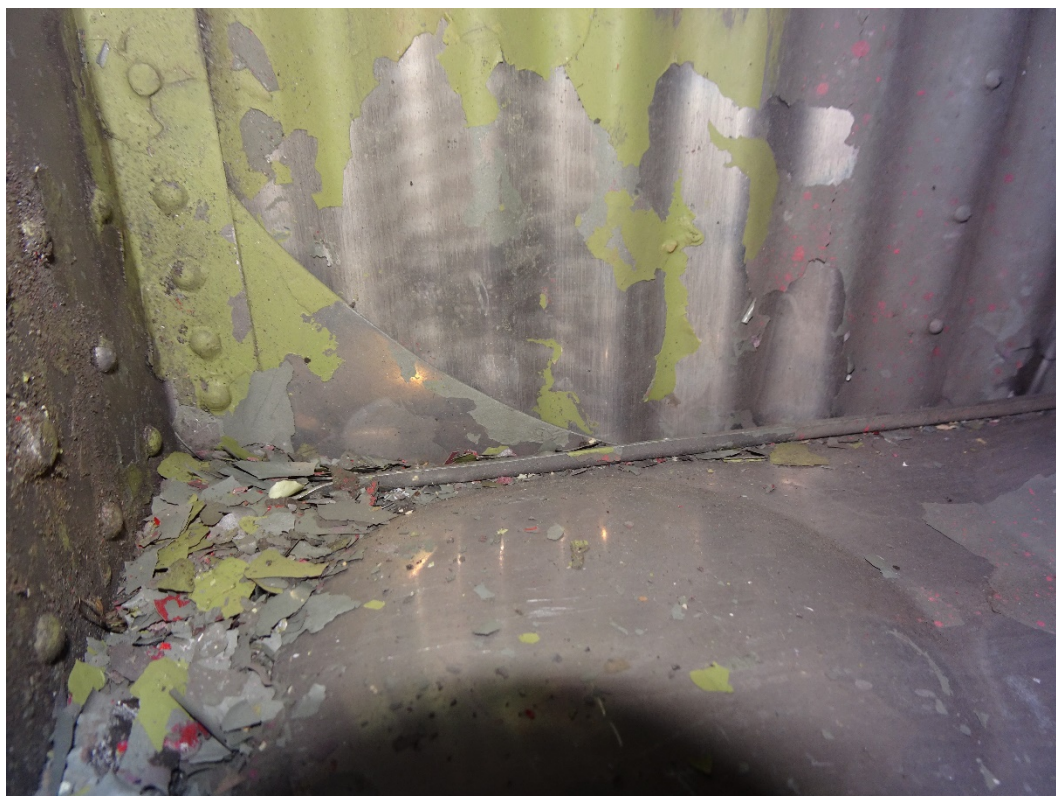
Figure 18: Flaked off anti-corrosion paint on the inside of the rudder.
