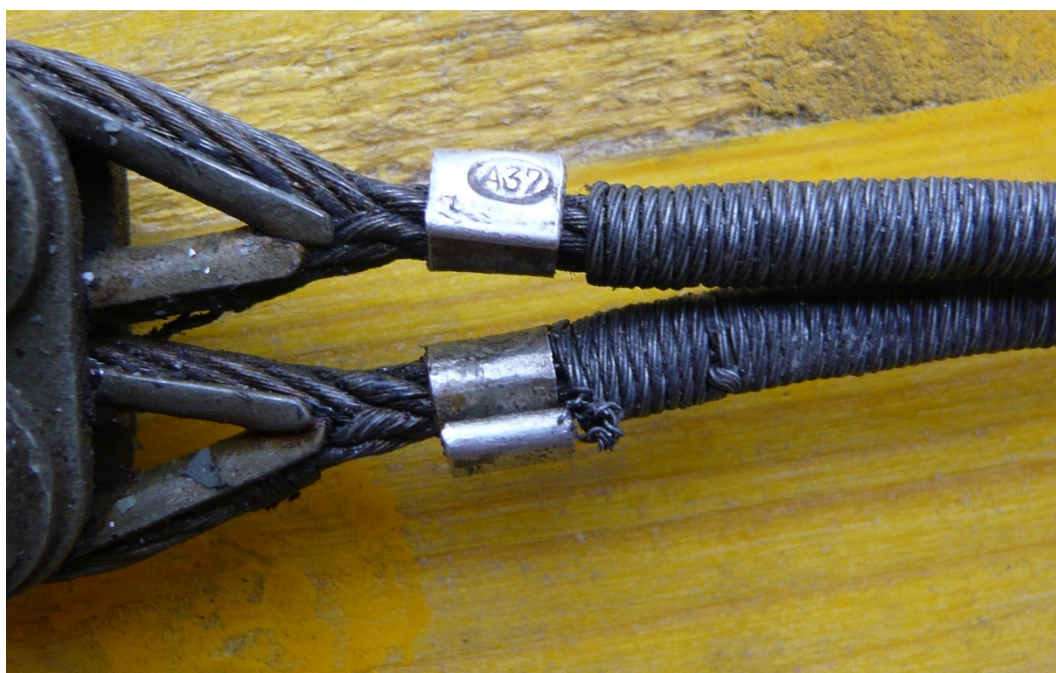
Figure 20: Old control cables, whose production method was consistent with the time when the aircraft was manufactured.
