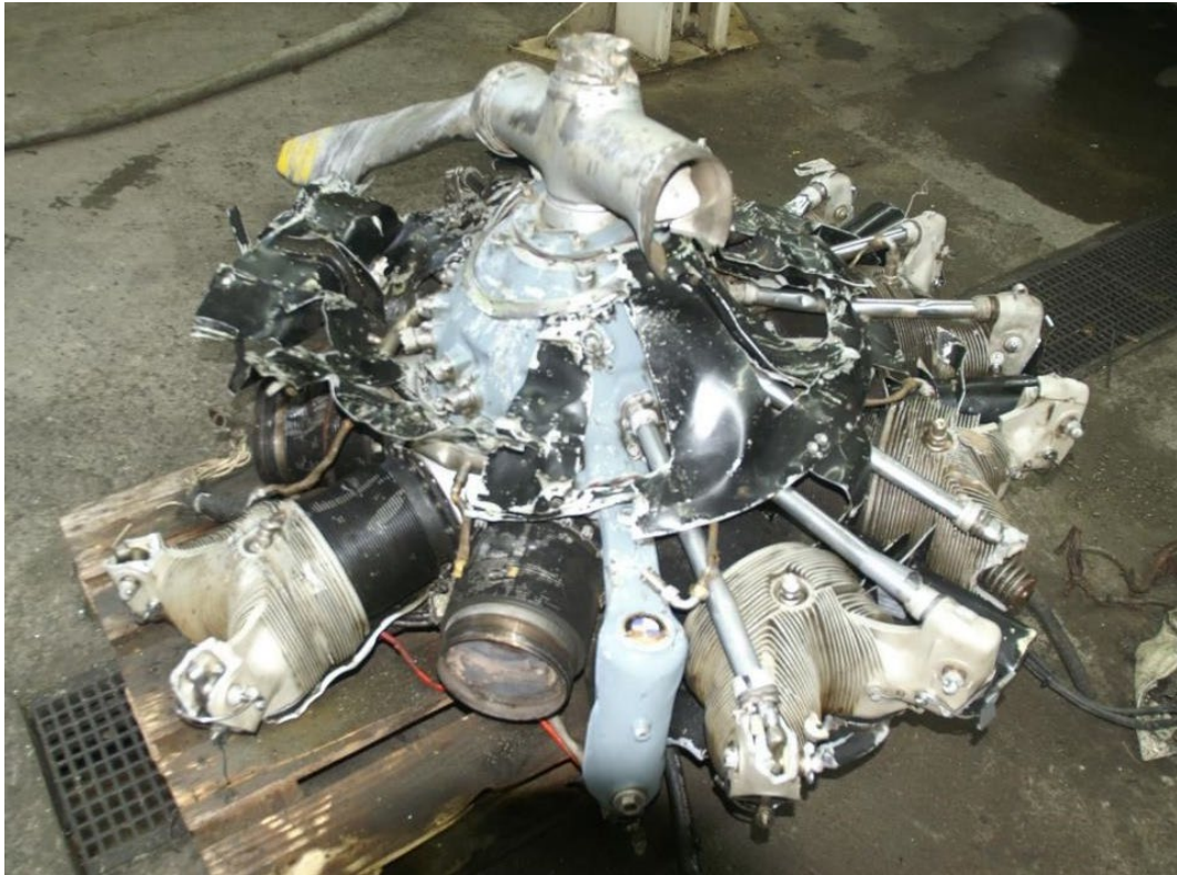
Figure 24: Engine cleaned using dry-ice blasting.
