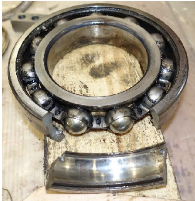
Figure 28: Broken outer race of the propeller bearing from the centre engine.
