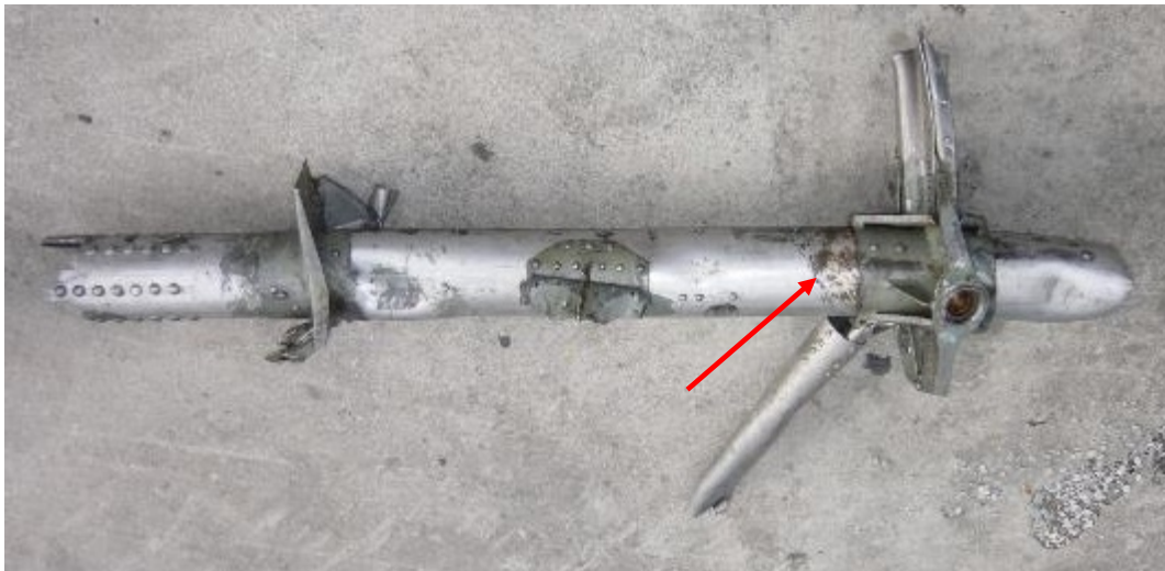
Figure 12: Lower spar tube of spar I on the left outer wing. The arrow points to the area of the spar tube with fractures. The outer diameter of the spar tube is 90 mm.
