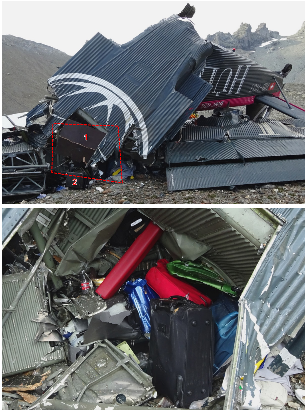
Figure 40: View of the HB-HOT wreckage – underside of the fuselage at the wing root, and luggage in the rear underfloor storage compartment.
