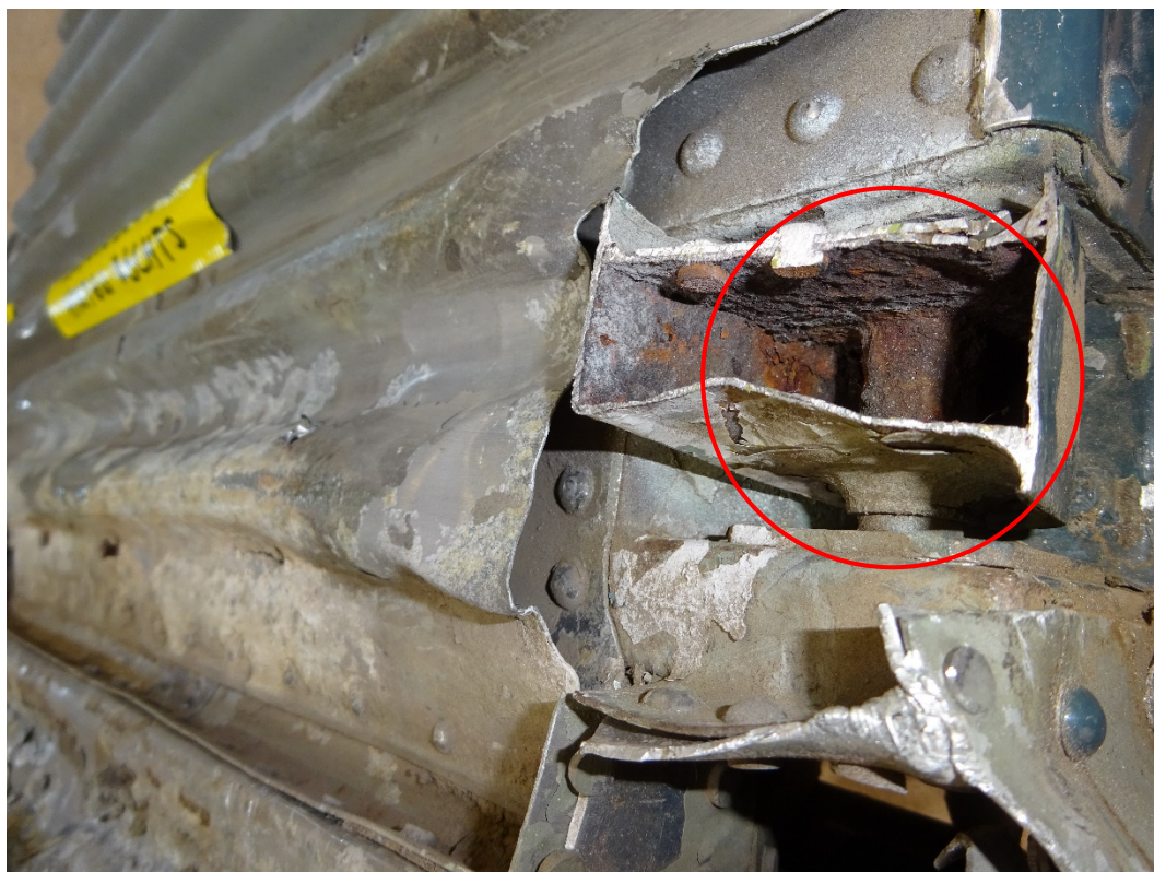
Figure 7: Close-up of figure 5 – severely corroded hinge of the cargo door (red circle).
