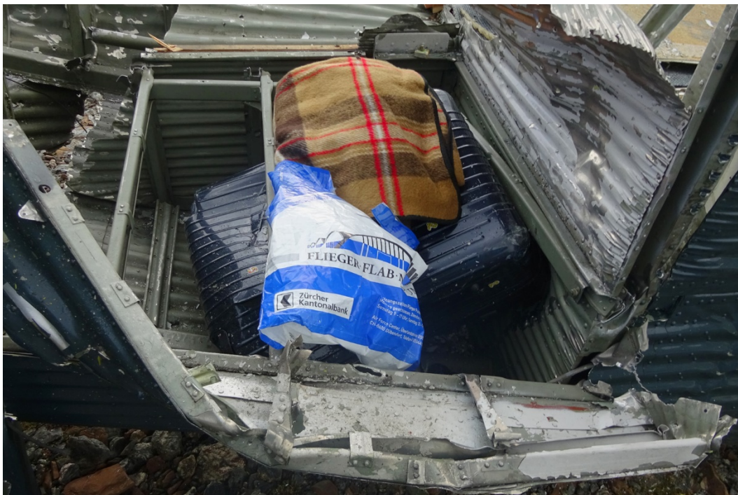
Figure 41: View into the fuselage structure below the toilet. A 15-kg dark-blue wheeled suitcase can be seen under a blue and white plastic bag and a brown woollen blanket. The wheeled suitcase ended up in this position after having moved from the front rear-storage compartment during impact.
