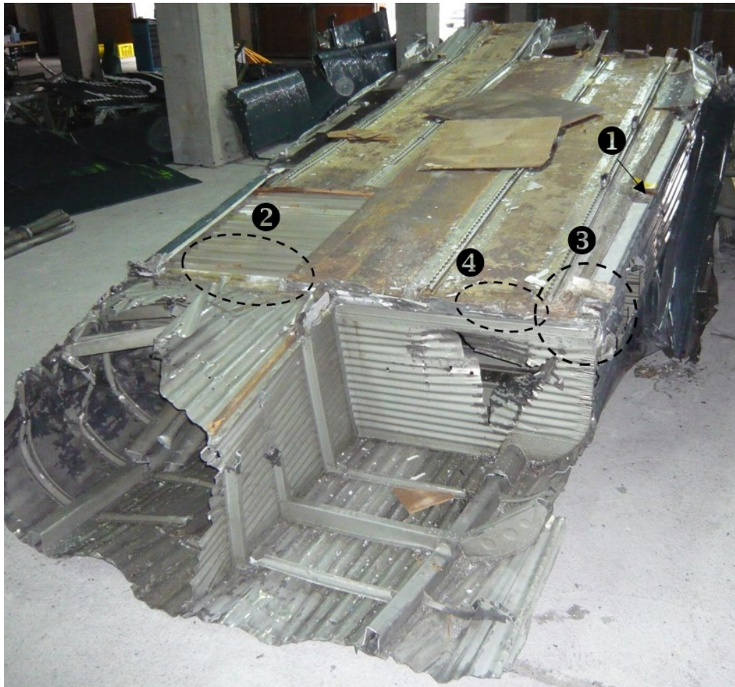
Figure 2: Aft bottom fuselage including cabin floor – severely corroded hinges of the cargo door (1) and (3), as well as severely corroded fuselage structure (2), (3) and (4).
