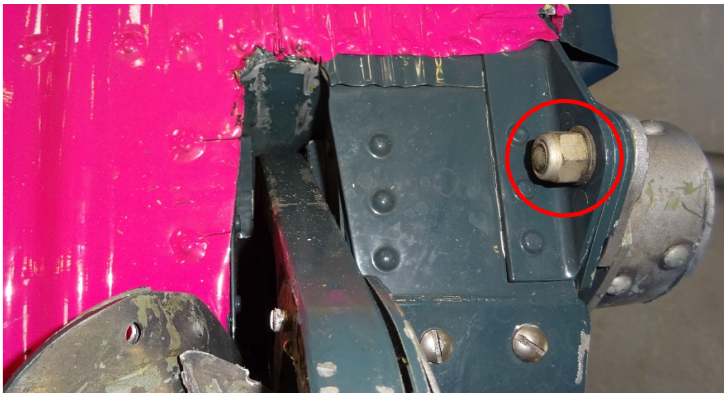
Figure 14: Right-side elevator with connecting flange of its actuating element, which was mounted using a nylon locknut on a thread that was too short for this purpose (red circle).
