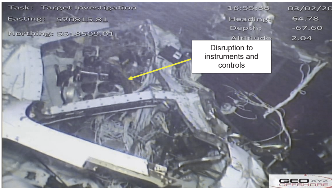
Figure B-11 Damage and disruption to instruments and controls
