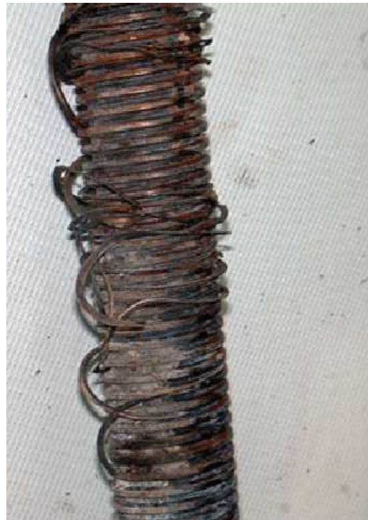
Figure 7 MD-83 horizontal stabilizer trim system jackscrew
