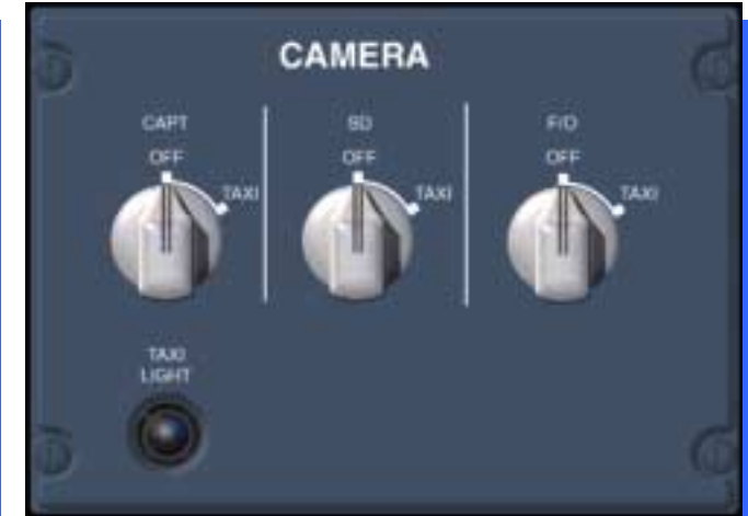
Taxi Aid Camera Control Panel
