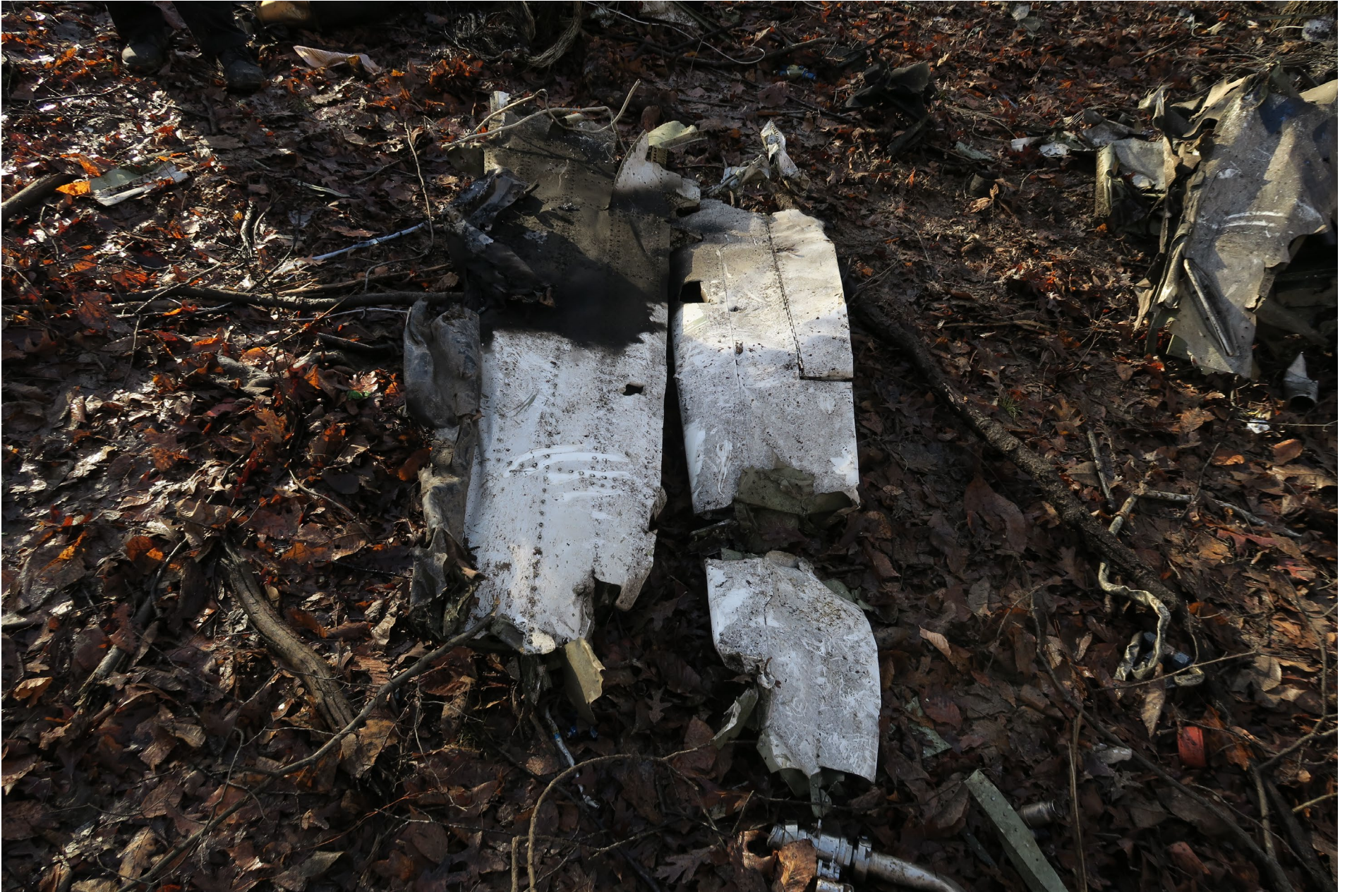
Photo 5 – Left Elevator Layout
