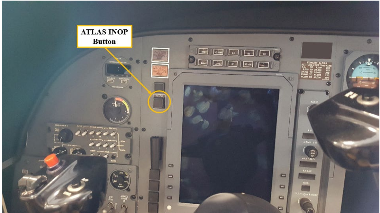
Figure 3 - Installation of the ATLAS INOP button in an exemplar aircraft (courtesy TAG)
