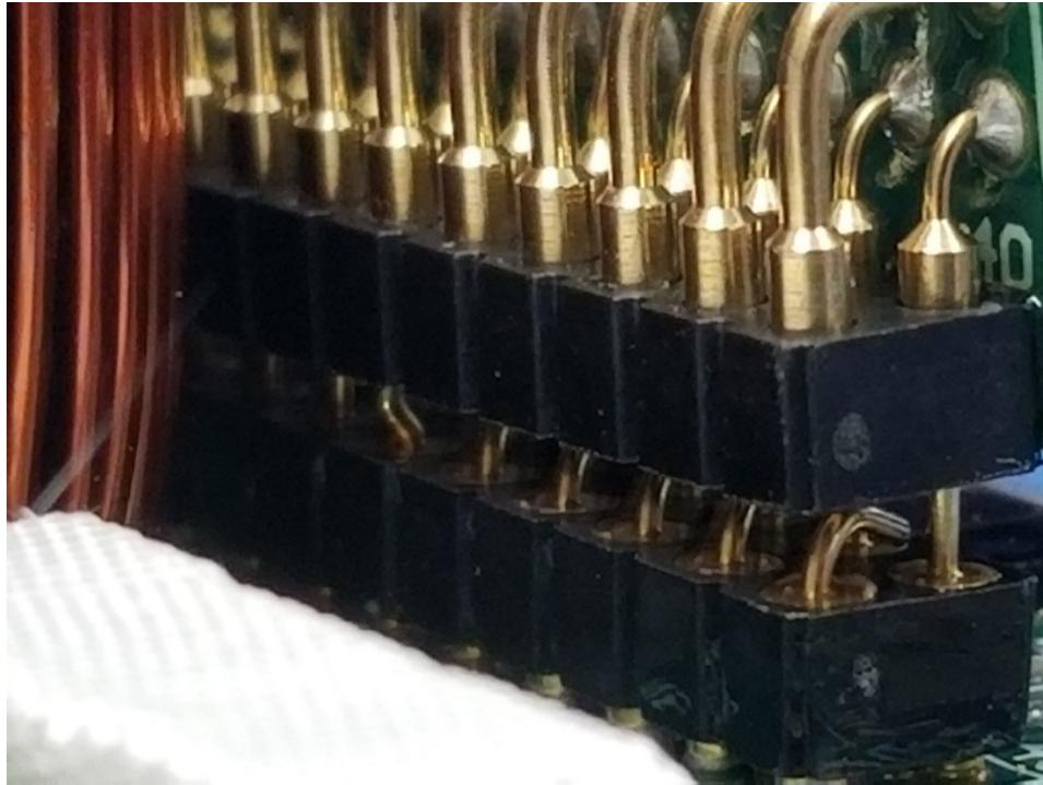
Figure 32 - View of the 40-pin connector showing damaged pins after center case removed
