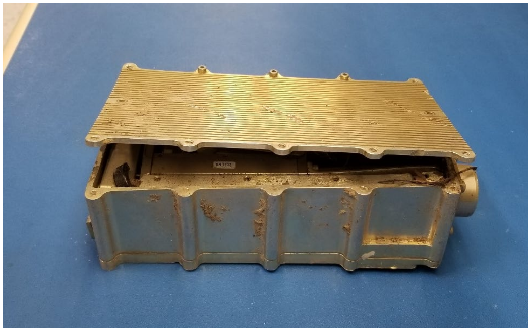
Figure 12 - RH TCU as recovered prior to visual inspection at the manufacturer
