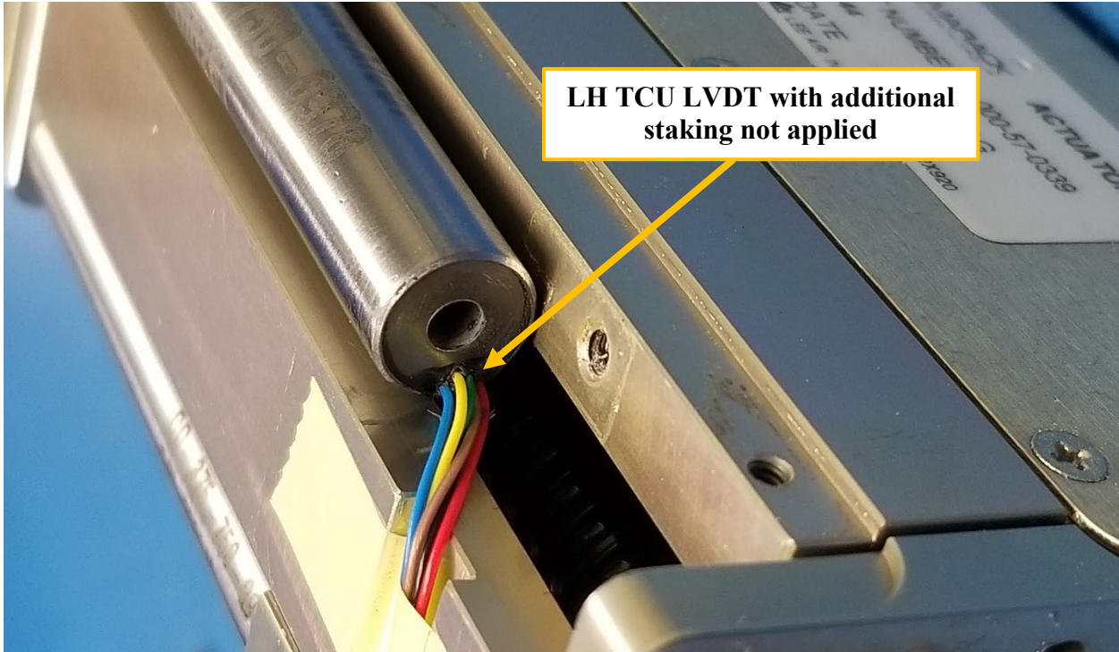
Figure 49 - One LVDT on LH TCU linear actuator
