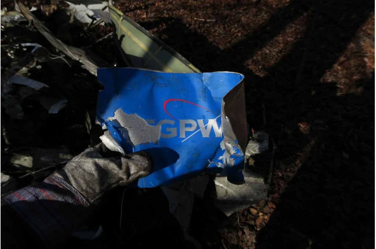
Figure 56 - Portion of outer cover of EGPWS unit (photo courtesy of Textron Aviation)
