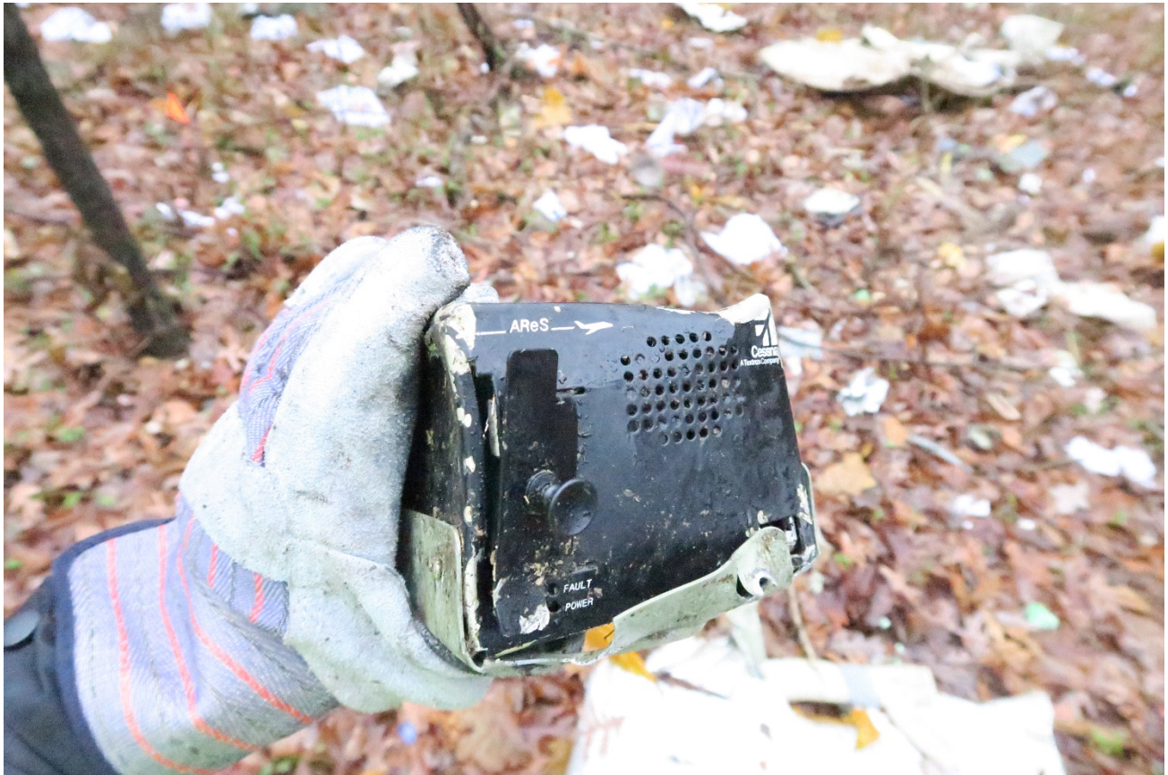
Figure 57 - AReS unit as recovered on-scene (photo courtesy of Textron Aviation)
