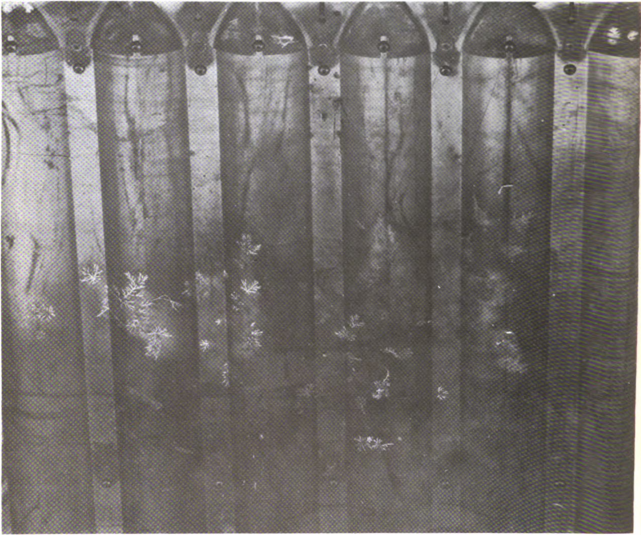
Figure 34. - Electrical arcing patterns on René 41 heat-shield surface.
