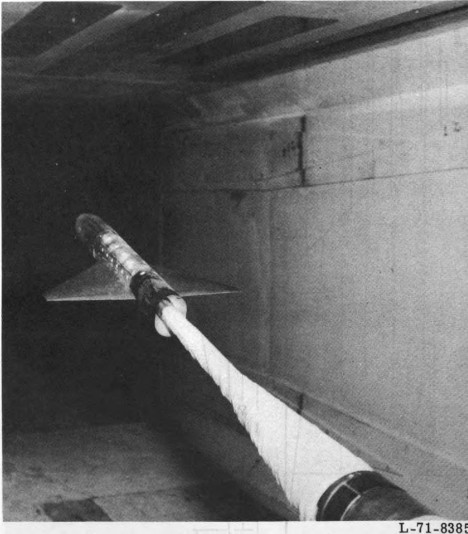
Figure 2.- Photograph of model in Langley high-speed 7- by 10-foot tunnel.
