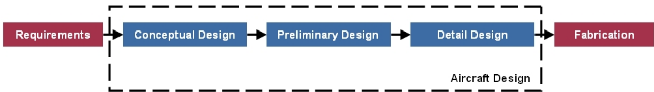
Figure 1.1: Three phases of aircraft design
