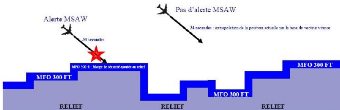
Figure 5: MSAW logigram (source: CDG Operating Manual)
