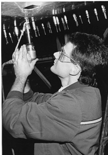
Photo 3. Usage of pneumatic tools in aviation maintenance. (Courtesy of Delta Air Lines)
