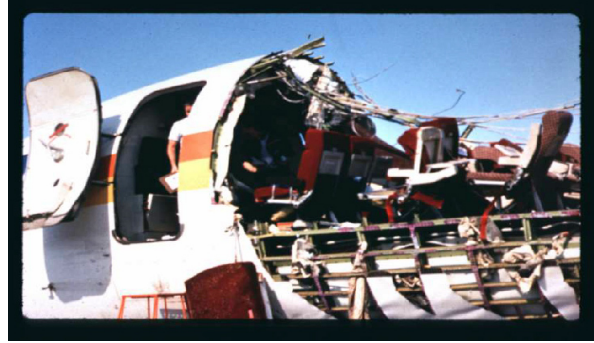
Photo 5. Aloha Airlines B-737 after skin de-lamination.
