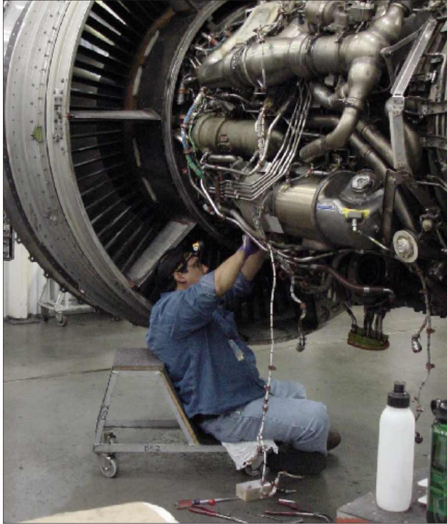
Photo 1. Working in an awkward position (note special rolling seat).
