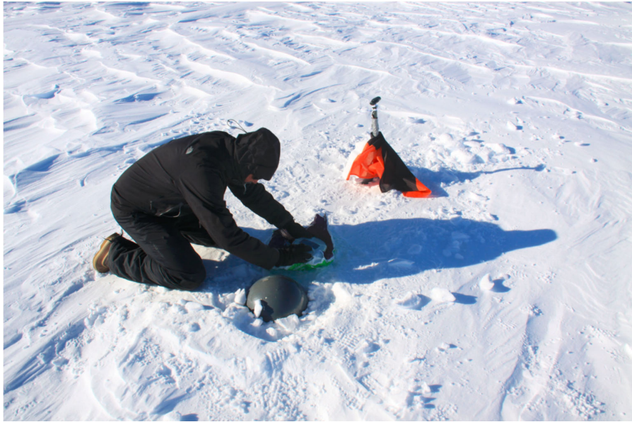
Fig. 47: GEUS member burying Luneburg sphere on ice sheet
