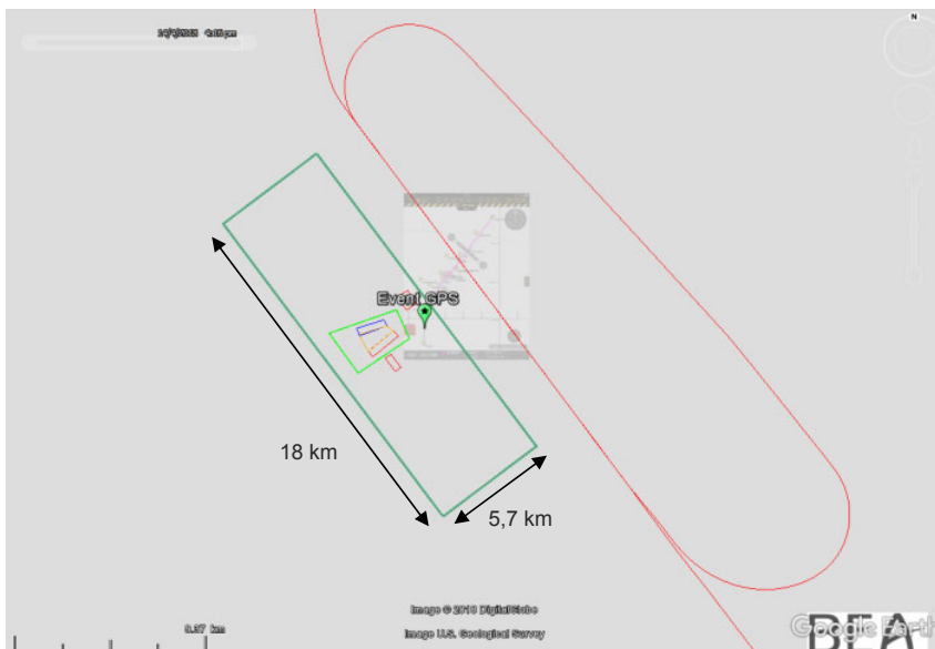
Fig. 67: UHF(P) and L band coverage and second flight trajectory for interferometric measurements
