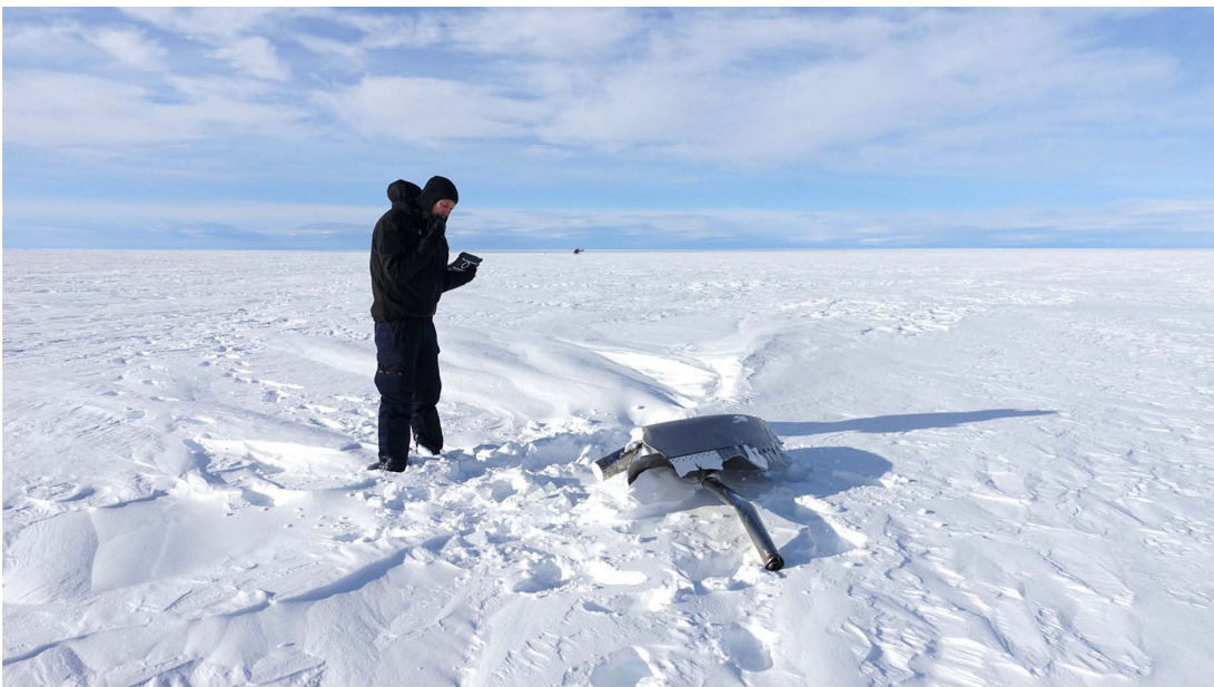
Fig. 7: part of inlet lip photographed on site by an Air Greenland staff member (picture courtesy of Air Greenland/AIB-D)
