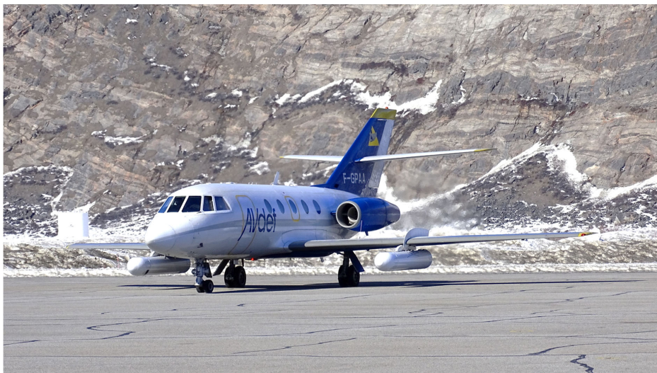
Fig. 68: Avdef Falcon 20 equipped with its two radar pods, back at Kangerlussuaq Airport
