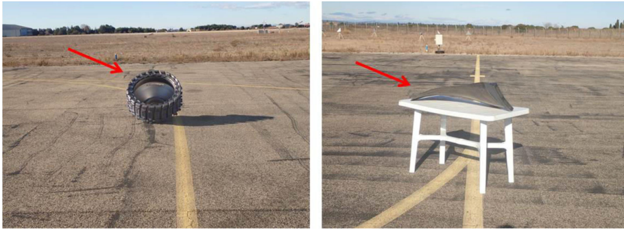
Fig. 41: a fan hub and a fan blade on Nimes-Garons airport for detection testing
