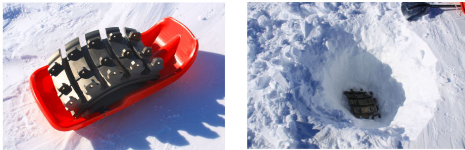
Fig. 48: part of a fan hub mock-up on its sledge, later referenced as “test hub” (left picture), and once buried (right picture)
