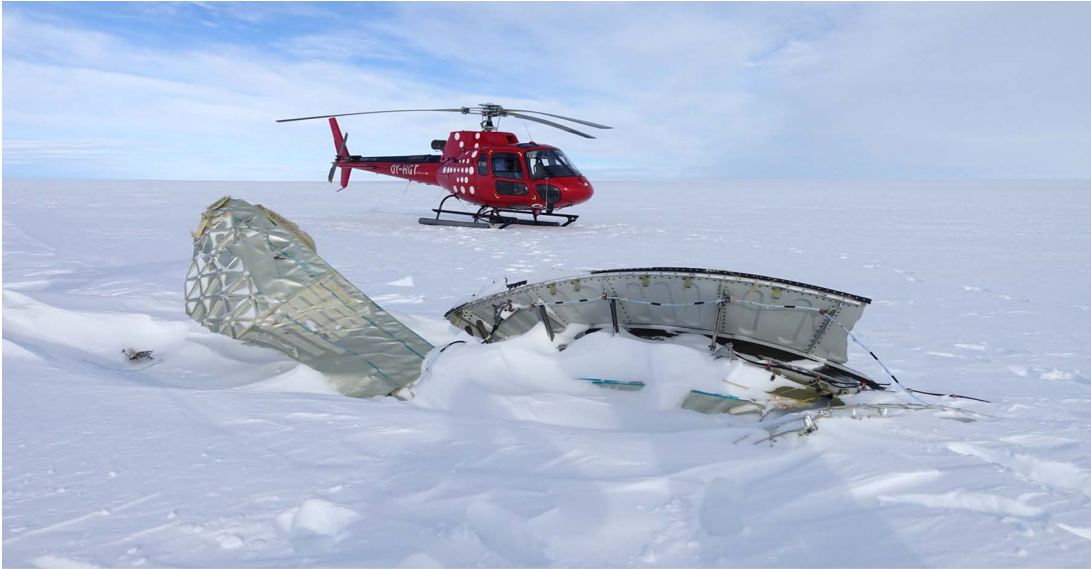
Fig. 6: bulkhead and fan containment case fragment as found on site (picture courtesy of Air Greenland/AIB-D)
