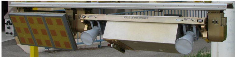
Fig. 39: X band radar payload (right) and L band (left) integrated in right pod
