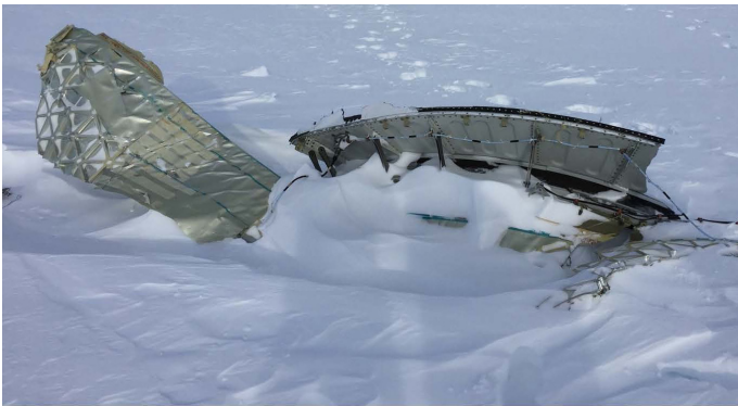
Fig. 10: inlet cowl aft bulkhead and fan containment case fragment
