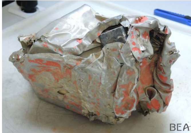
Initial state of the CVR
