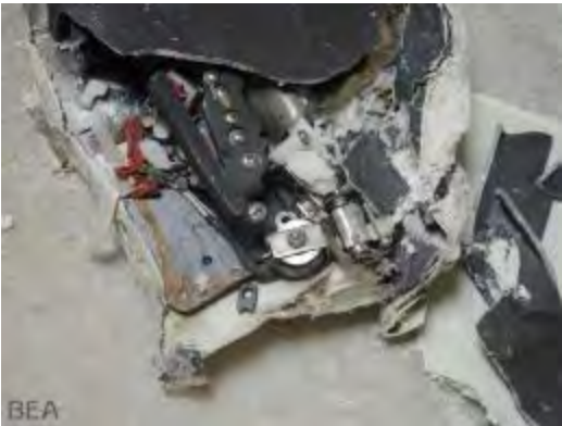
Figure 33 - Close-up - magnetic tape mechanism extraction
