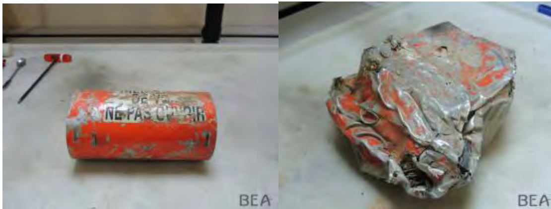
Figure 24 - FDR protected module (on the left) and CVR (on the right)
