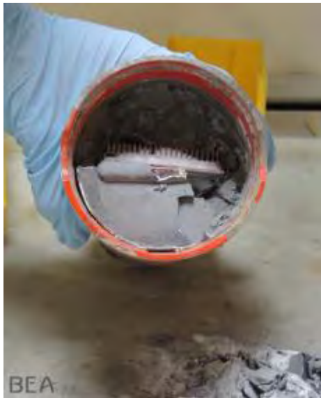
Figure 25 - Electronic card in the CSMU
