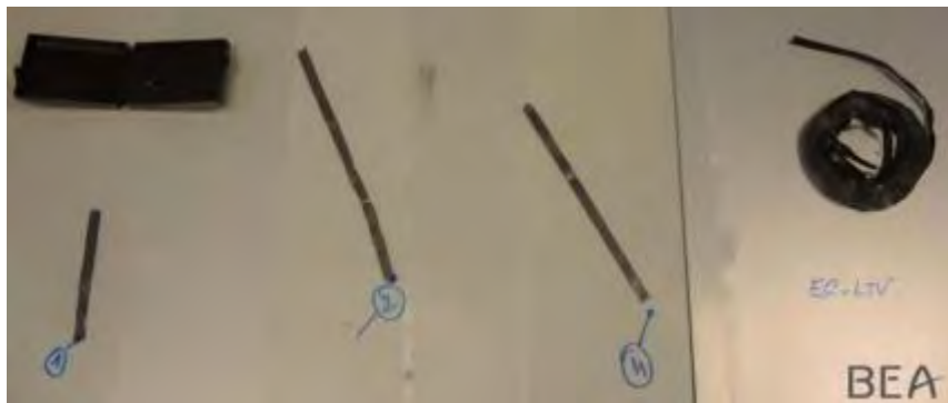
Figure 35 - Sections of magnetic tape recovered during the opening operations
