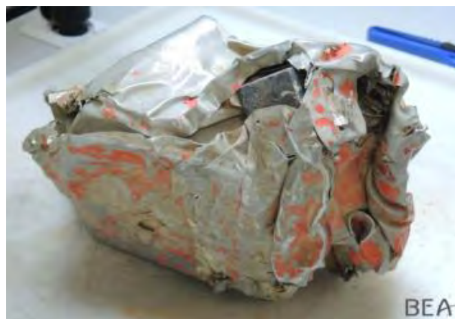
Figure 28 - Initial condition of the CVR
