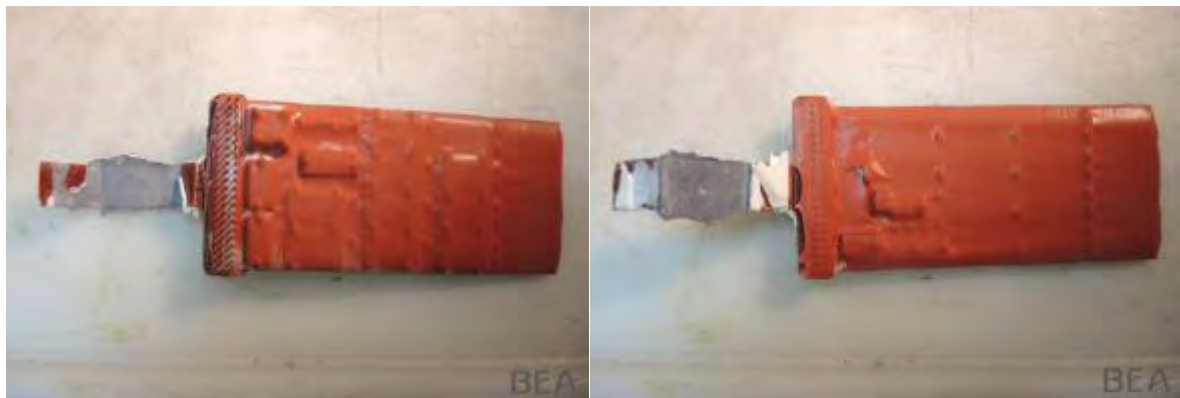
Figure 26 - Electronic card with the protective layer
