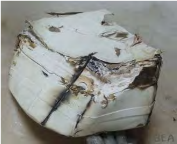
Figure 31 - Data carrier heat protection
