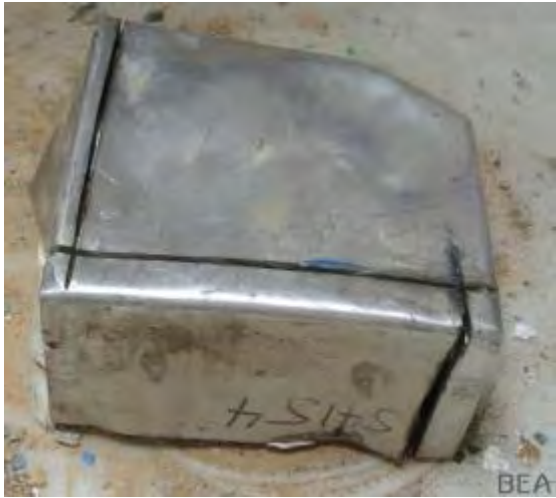
Figure 30 - Protected module after extraction
