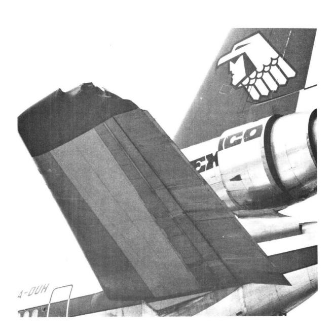
Figure 1.--View of left outboard elevator tip.
