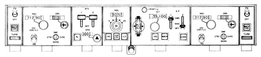
Figure 3.--Flight guidance and control system panel.
